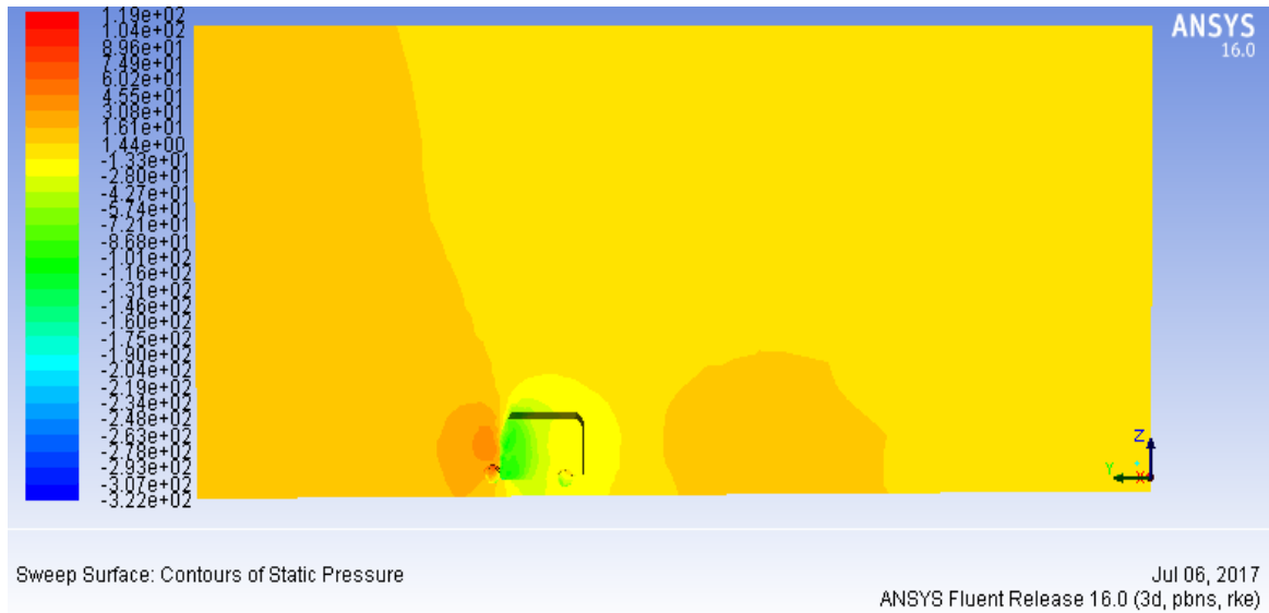
Figure 48: Pressure Distribution of Model 2 at 50 Km/h
