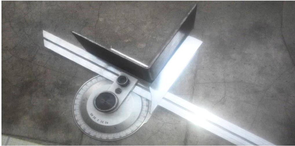
Figure 3. 4: Measuring the angle of bended sample
