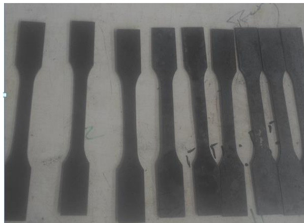
Figure 3. 12: Specimen prepared for tensile test
