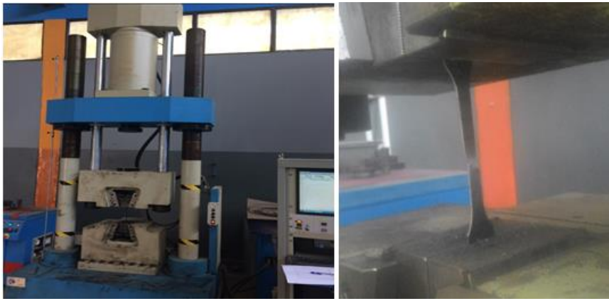
Figure 3. 13: Tensile testing by using UTM-2000kN
