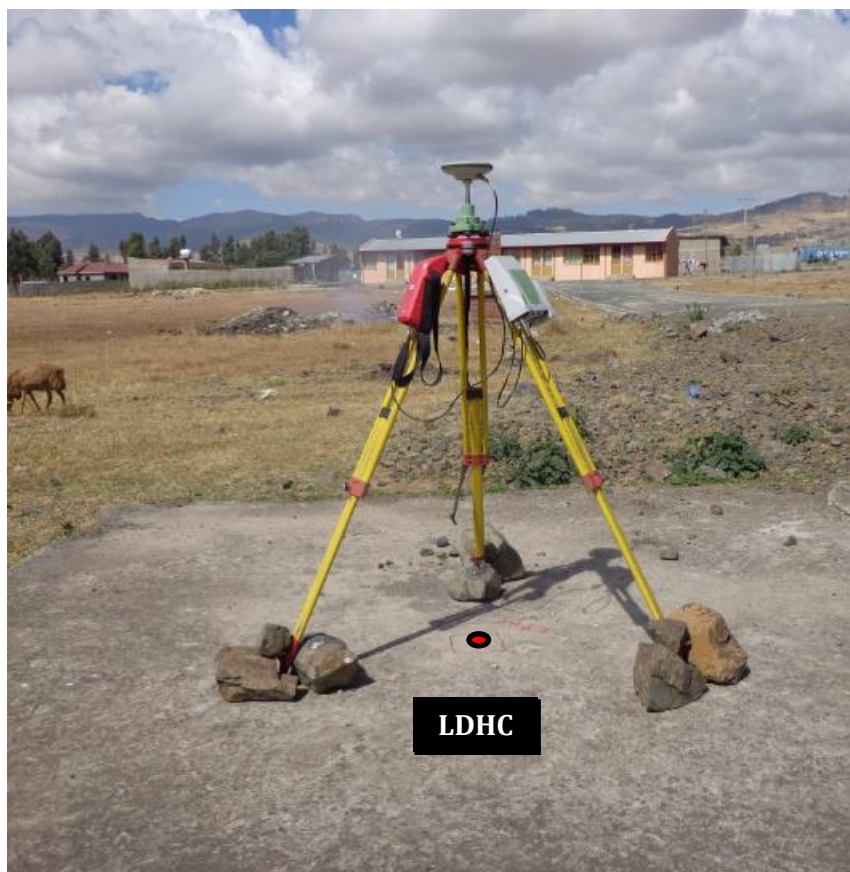
Figure 3. 3: Leica GS10 GNSS receiver observing data at station LDHC.
