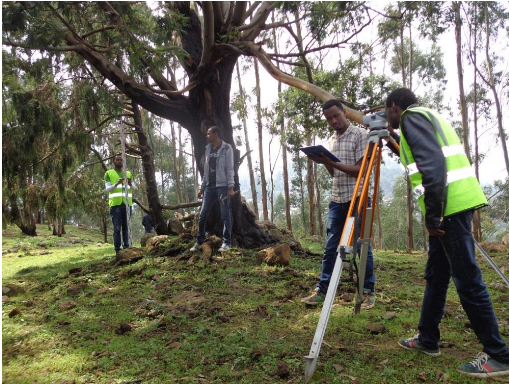
Figure 3. 4: Levelling crew conducting differential levelling.
