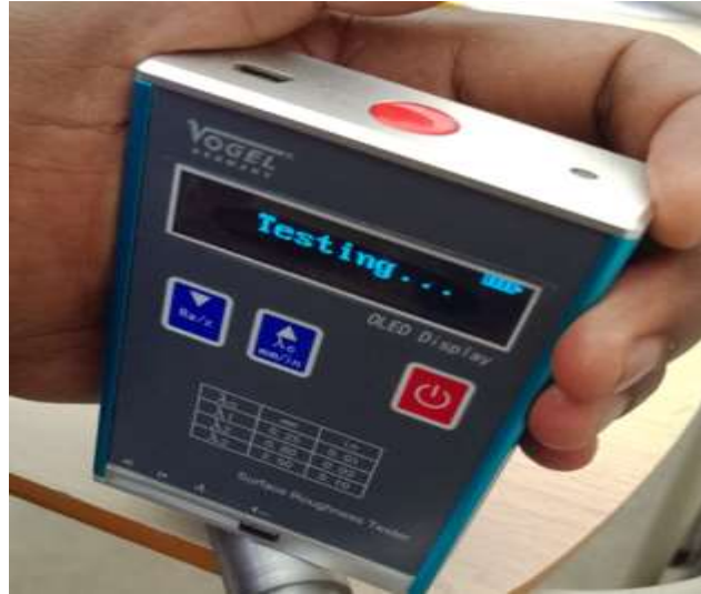
Figure 3. 8 Profilometer Measurement of Surface Roughness Device
