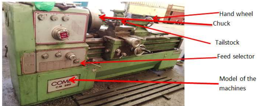
Figure 3. 6 Conventional Lathe Machine used for Experimental Work
