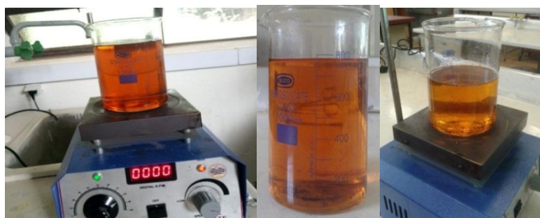
Fig.3.14. heating and drying biodiesel
