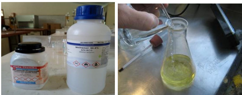
Fig.3.2. Methanol and potassium hydroxide and measuring KOH & dissolve it in methanol
