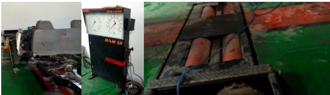
Fig.3.18.chassis dynamometer and checking its working vehicle performance test
