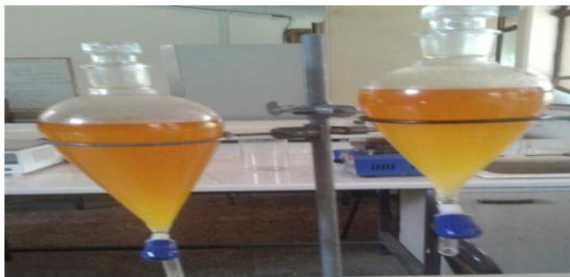
Fig. 3.8 washing of biodiesel with distilled water.
