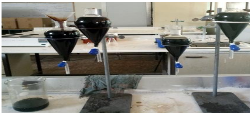
Fig.3.5. the heated mixtures of KOH & methanol) with crude oil was poured into the reparatory funnel
