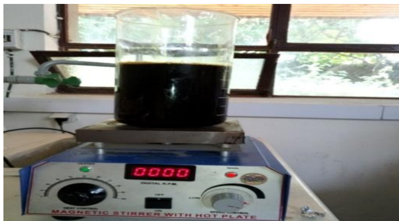
Fig.3.4. Heating the mixtures of KOH & methanol) with crude oil.
