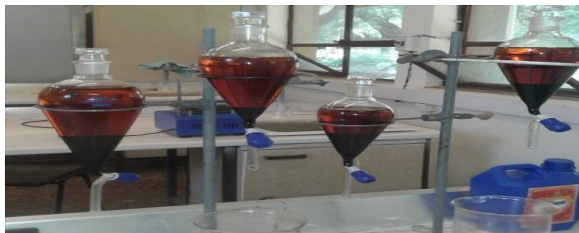
Fig.3.6 Two layers of oil formed
