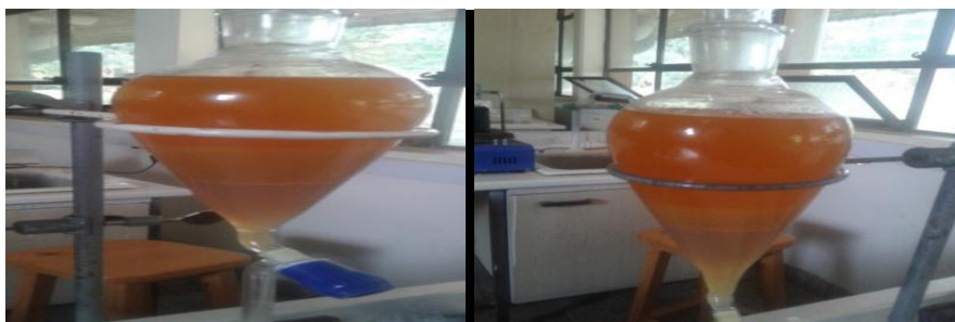
Fig.3.9. 1 st step washing of biodiesel with distilled water (soap formation)
