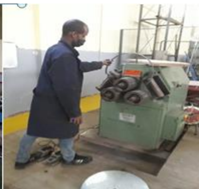
picture showing rolling ring on roller Machine at ARIC work shop
