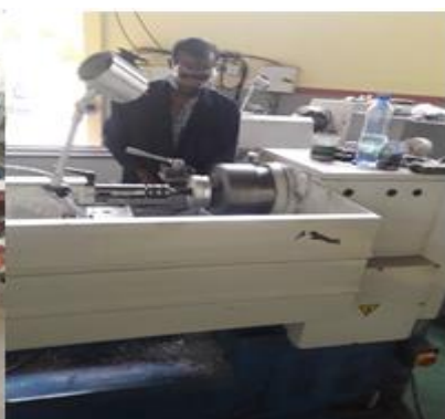
picture showing pulley manufacturing at ARIC Work shop using lathe machine
