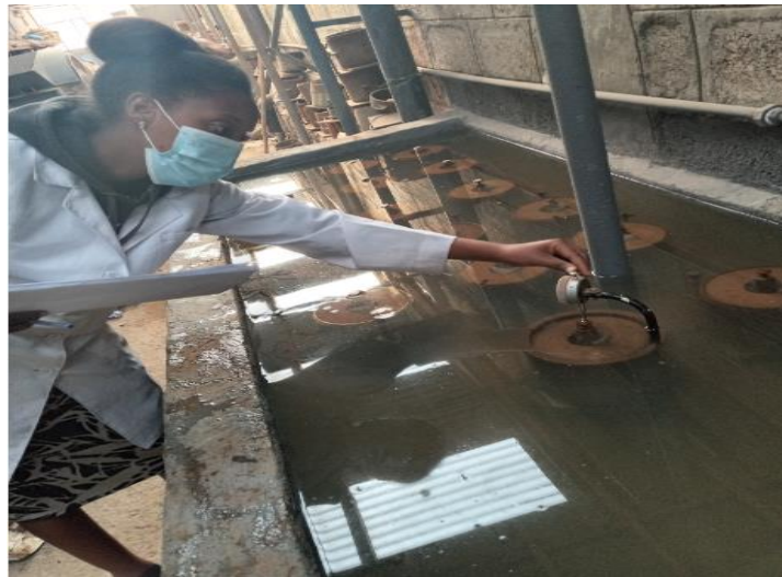
Figure 3. 8 CBR samples in a soaking condition
