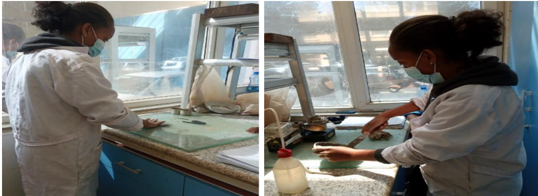
Figure 3. 7 Photographic views of plastic limit and liquid limit test
