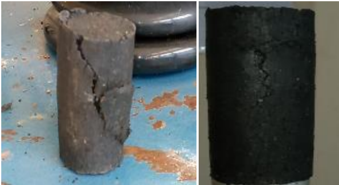
Figure 3. 9 UCS specimens after testing until failure
