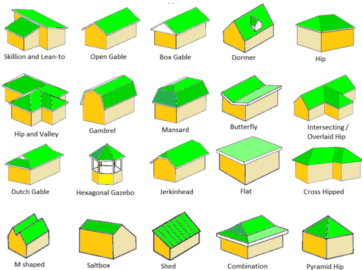
Figure 3: Roof types (Maghiar et al., 2020)
