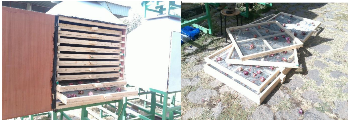
Fig. 34 Onion after drying in solar drier
