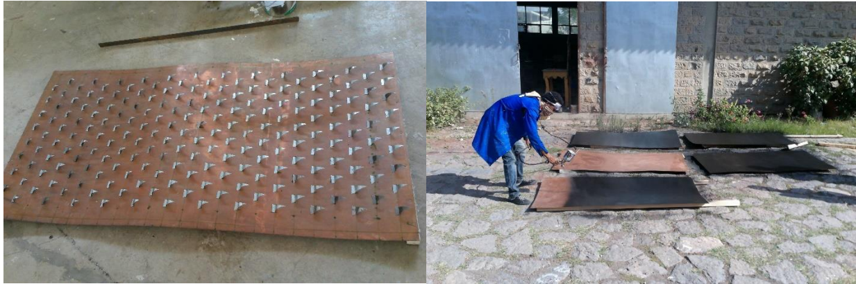
c) Tabulators fixed and the absorber plate is black painted to maximize solar absorption
