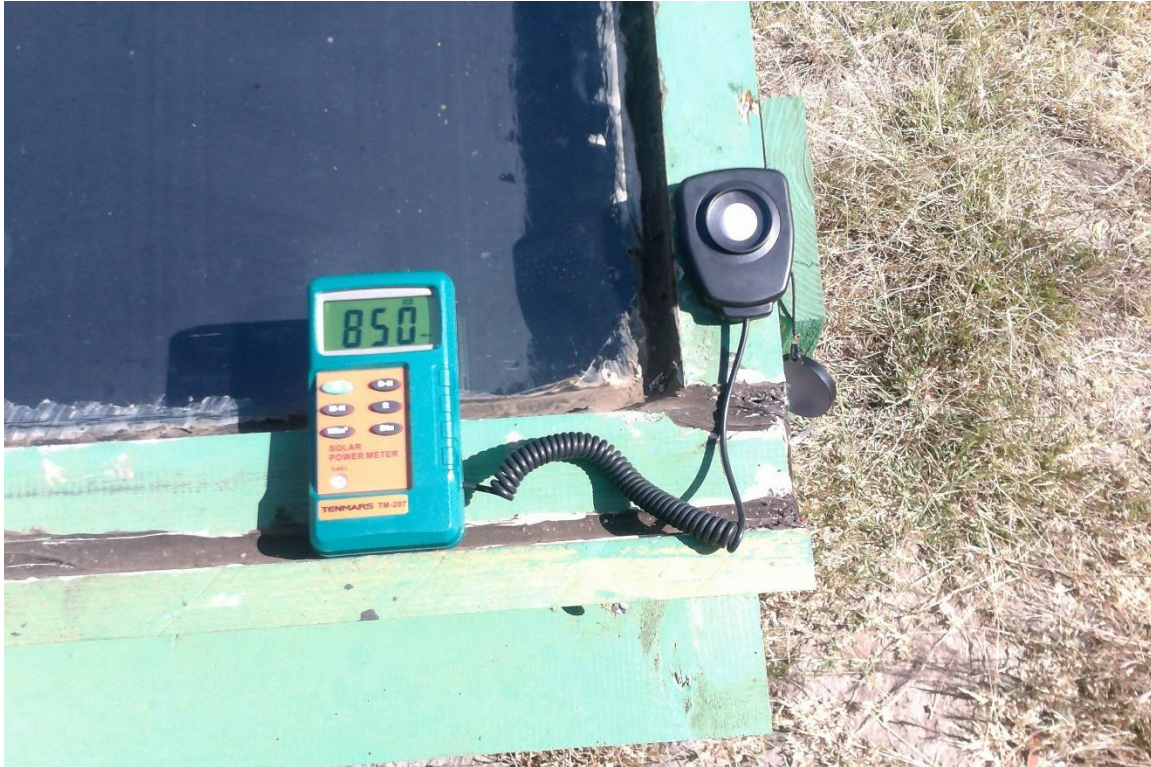
Fig. 16 Solar Power Meter used to measure radiation during testing of the solar drier
