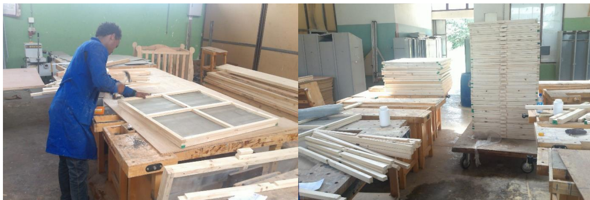
b) Manufacturing of tray of the drier using galvanized wire mesh
