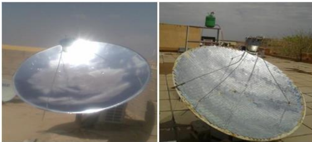
Figure 2.10: Parabolic dish concentrator for water heating purpose (Yaseen et al. , 2018).
