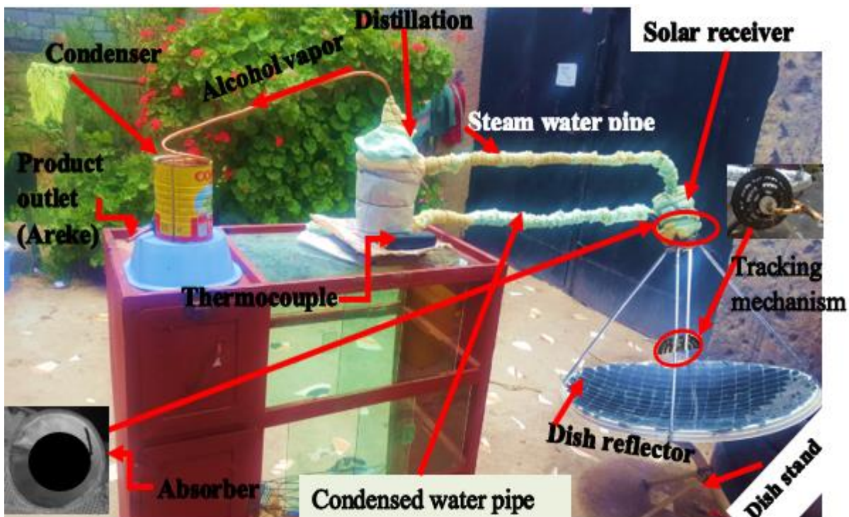
Figure 6.1: Experimental setup of solar thermal Areke production system.
