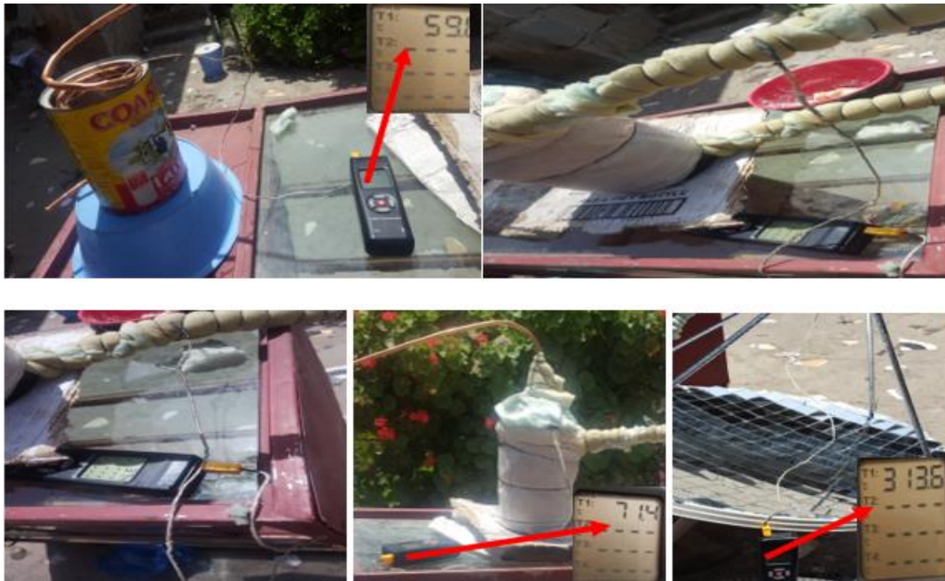
Figure 6.2: Thermocouple installation on each component.
