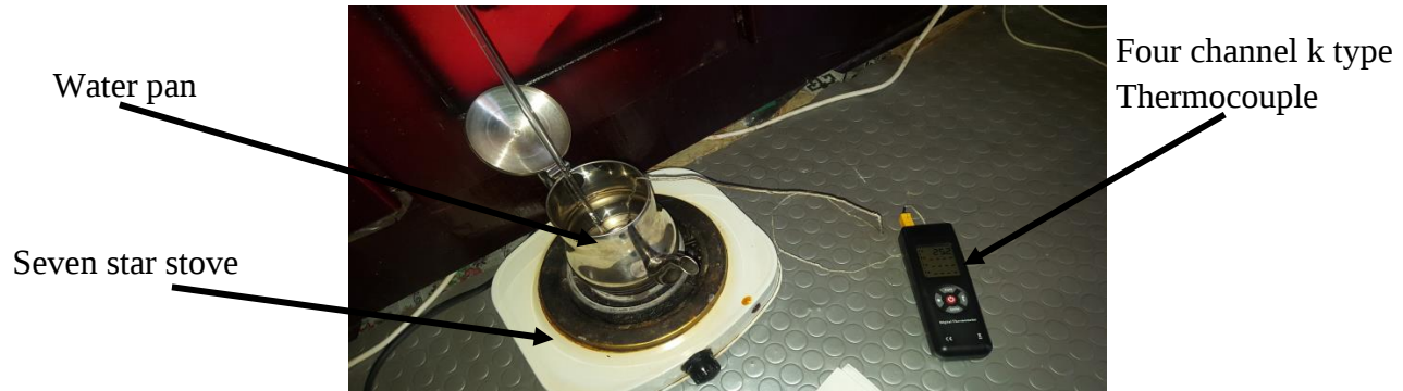
Figure A. 1: Calibration Setup.
