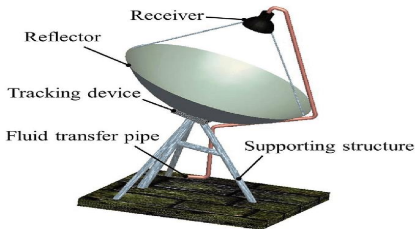
Figure 2.2: Parabolic dish collector (Pushkaraj et al. , 2017).
