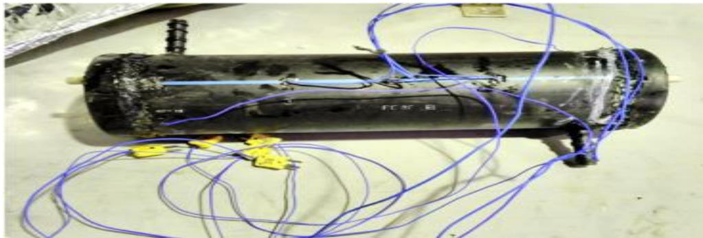
Figure 2.14: Shell and coil heat exchanger (Ashkan 2017).
