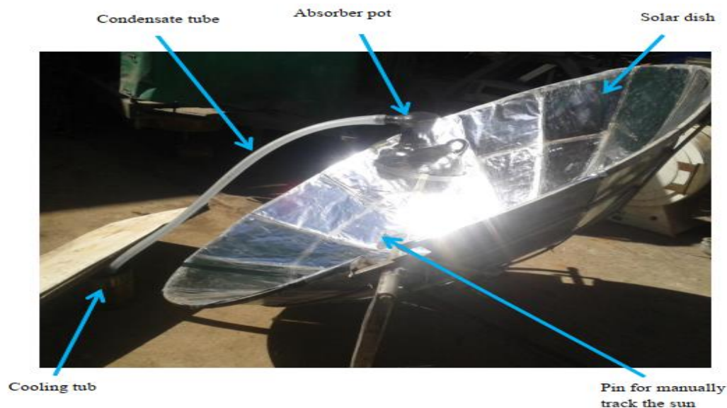
Figure 2.9: Direct solar thermal Areke distillation (Adane, 2015).
