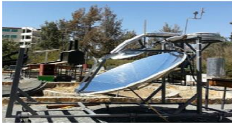
Figure 2.13: Solar thermal injera baking stove (Asfaw et al., 2014).
