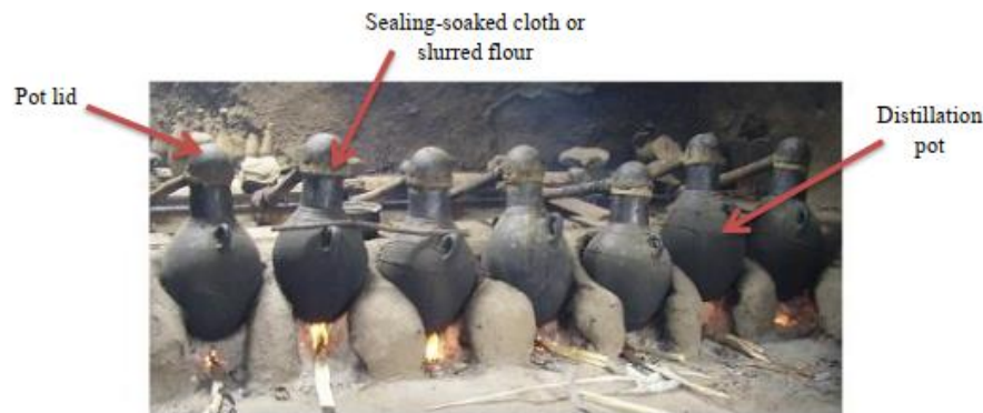
Figure 3.4: Traditional distillation stove (Girma, 2008).
