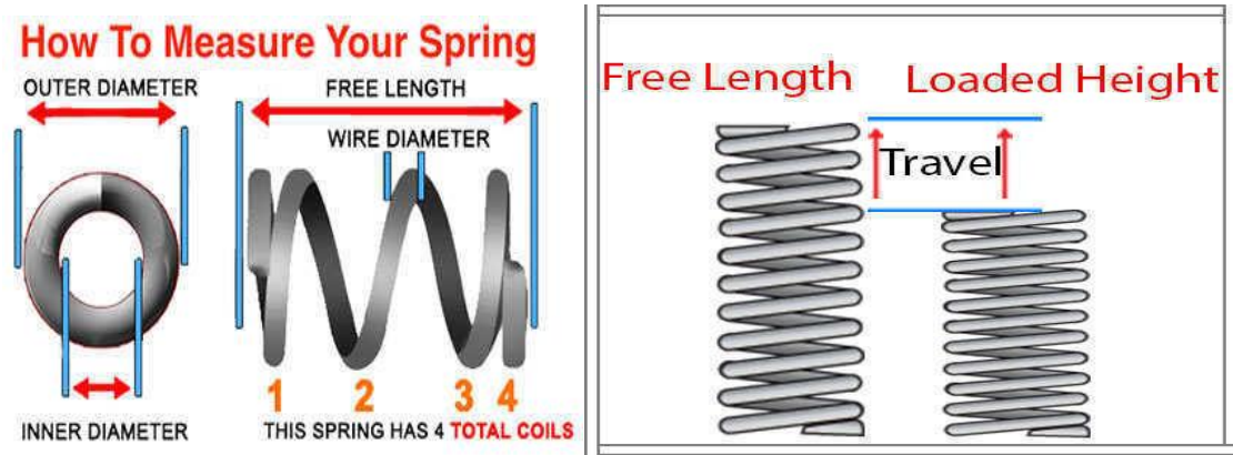
Figure 3.9 Dimension of compression spring (Spring Engineers of Houston, Ltd.) http://www.springhouston.com )
