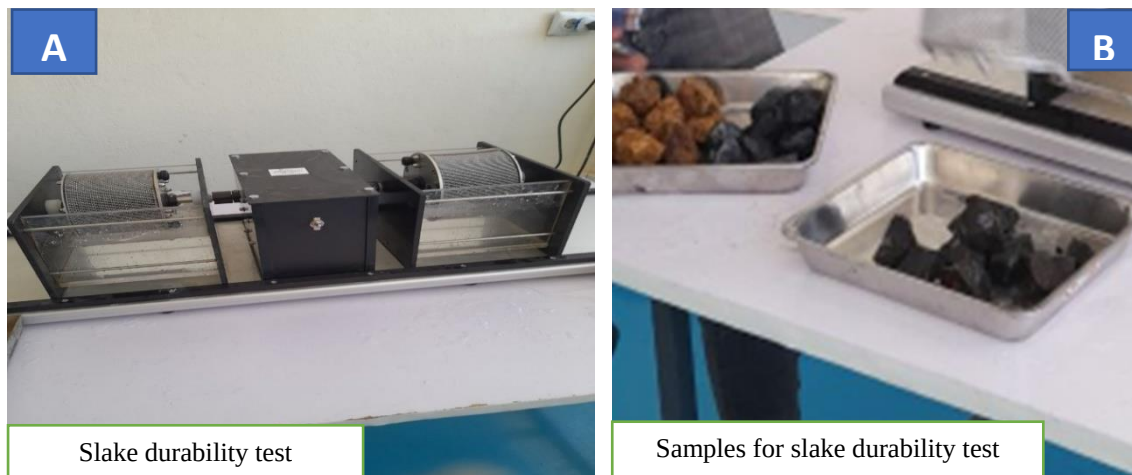
Figure 3.6 slake durability test, A) slake durability apparatus B) 10 rock samples for the slake durability test
