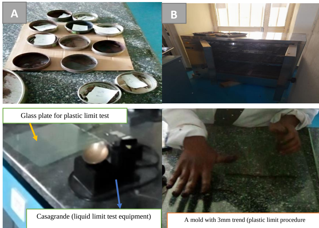
Figure 3.5 Methodology for Atterberg test, A) samples for LL and PL test, B) oven for water content determination
