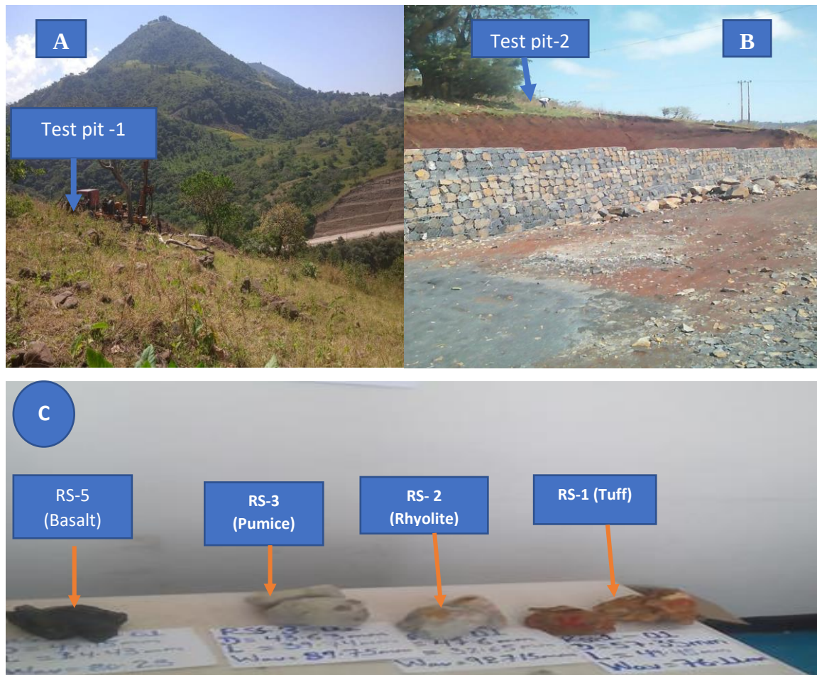
Figure 3.1 Sample collection A) soil sample collection from test pit-1, B) soil sample collection from test pit-2, c) rock sample
