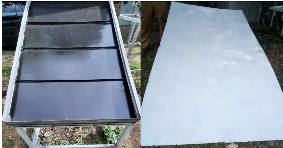
Figure 5. 1: View of a) solar collector from the inlet side b) anti-rust painted absorber plate
