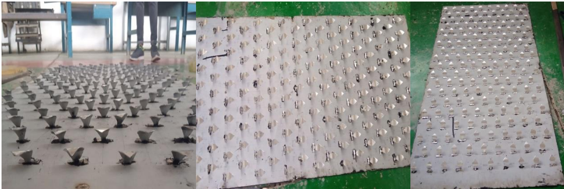
Figure 5. 4: Photographic view of the absorber plate with spoon-shaped obstacles mounted for e/H = 0.50 at an angle of attack 30^\circ
