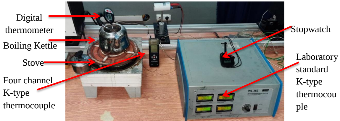
Figure B- 1: Calibration setup with standard and K-type thermocouples
