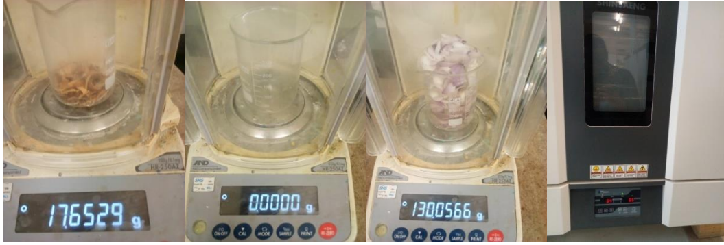
Figure 4. 8: Laboratory experimentation devices to measure moisture rate a) Digital weight balance calibration b) mass of onion before drying c) mass of onion after drying d) oven dryer
