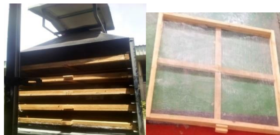
Figure 5. 2: Construction of the drying chamber with a tray
