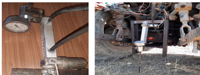
Figure 3.4: The integrated cone penetrometer on the tractor
