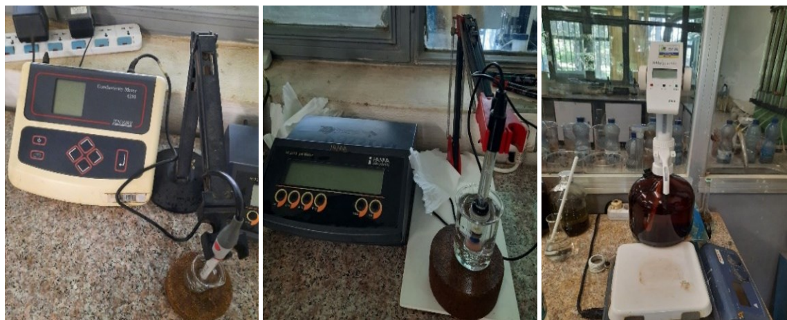
Figure 3.11: a) soil pH, b) soil electric conductivity, and c) soil organic content test
