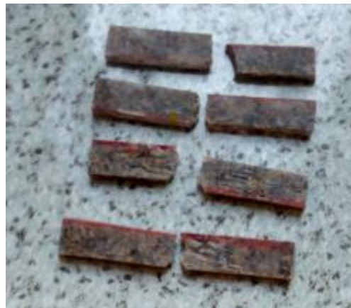
Fig. 3.15 Some of the failed specimens during an impact test
