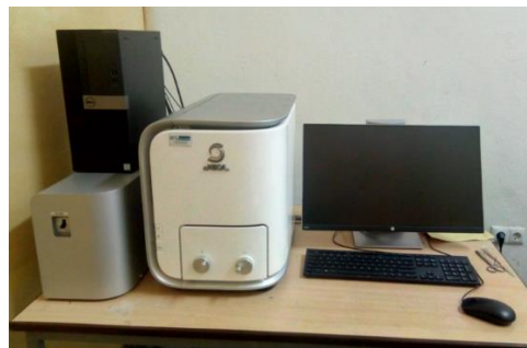
Fig. 3.18 JCM-6000Plus scanning electron microscope (ASTU biology laboratory)
