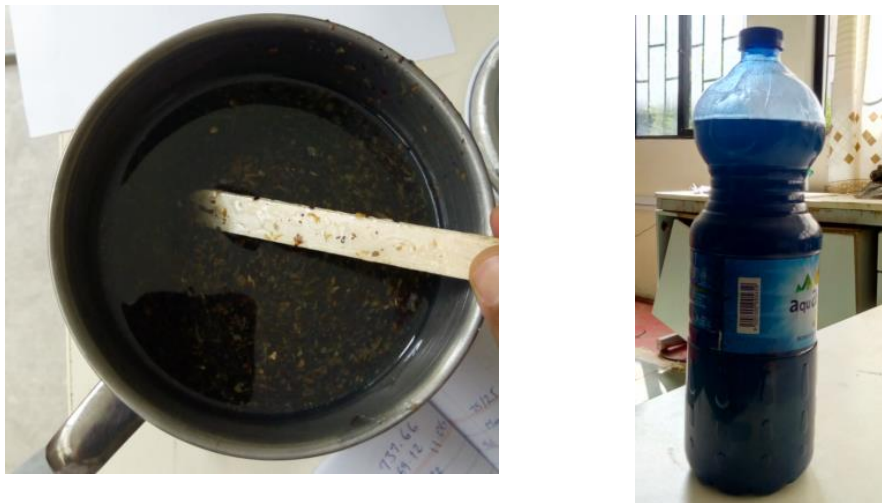
Fig. 3.6 a) mixing coffee husk and polyester b) unsaturated polyester resin
