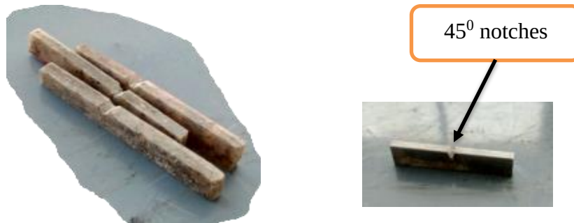
Fig. 3.14 Prepared impact samples and 45-degree notch guide tool
