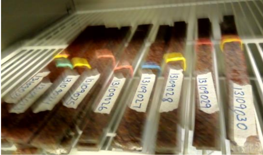
Fig. 3.11 Prepared tensile samples under controlled environment
