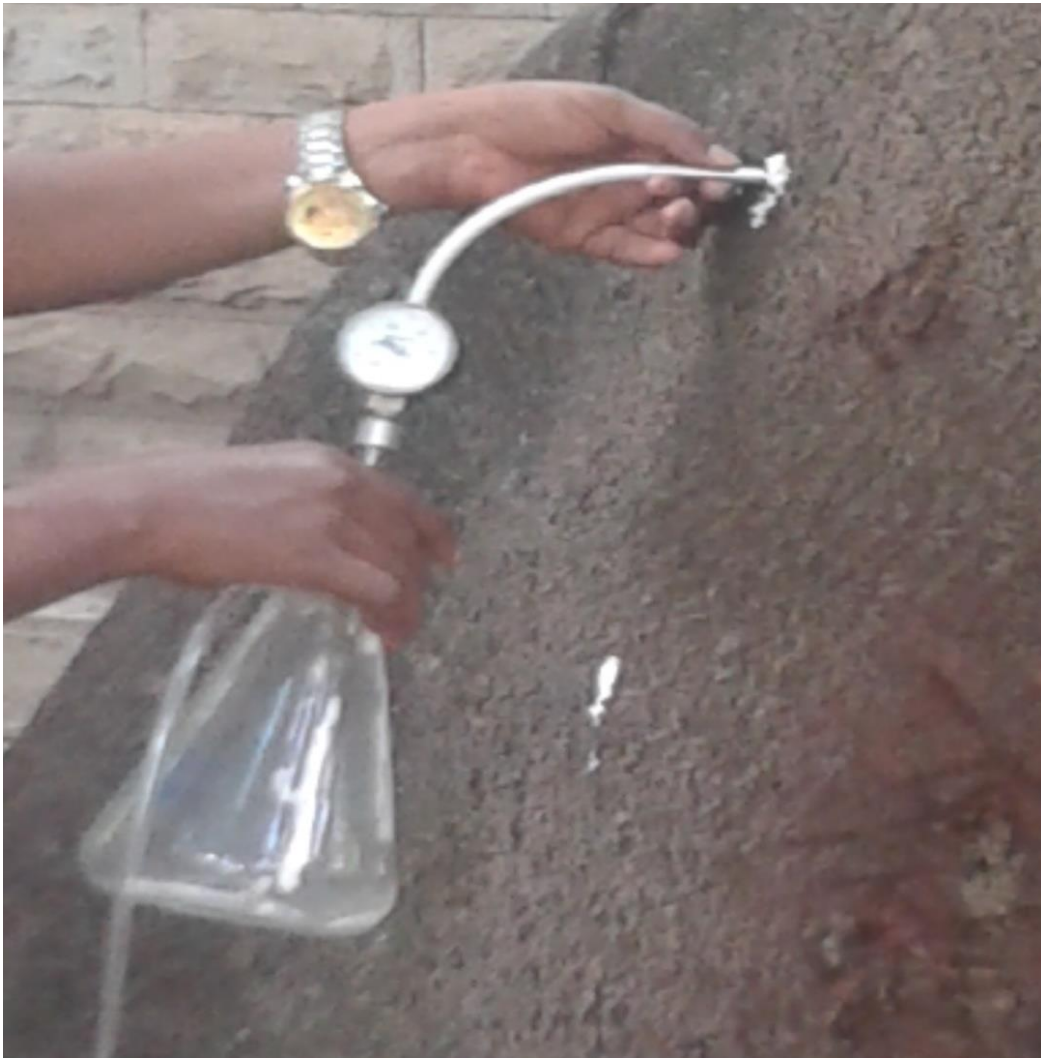
Figure 4-23 Extraction of Phytochemicals from Holes Made by Large Needle
