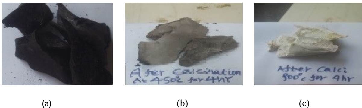
Figure 4. 5 Bone char image after calcination at different time and temperature a) 300°C, 1 hr b) 450°C, 4 hr and c) 900°C, 4 hr.
