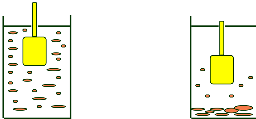
Figure 2.2 A schematic view of the hydrometer test [11]
