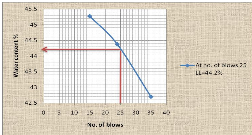
Figure 4.6 Liquid Limit plot for Bargale soils
