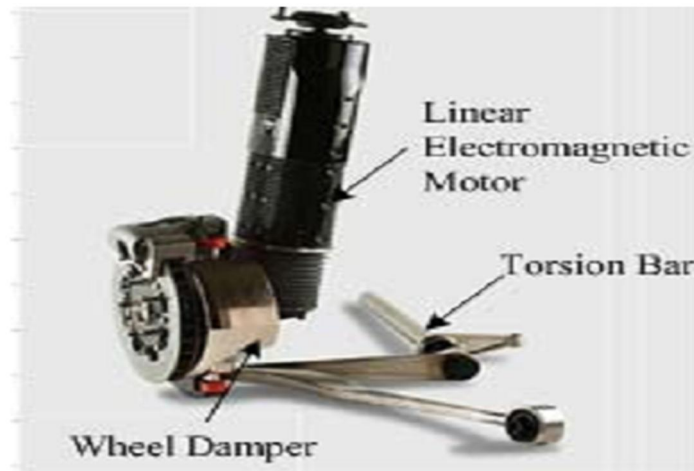
Figure 2.8: Electromagnetic suspension developed by Bose
