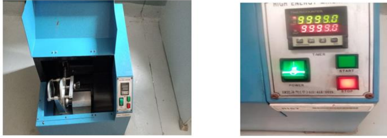
Figure 3.4 Photos of High Energy Planetary Ball Milling
