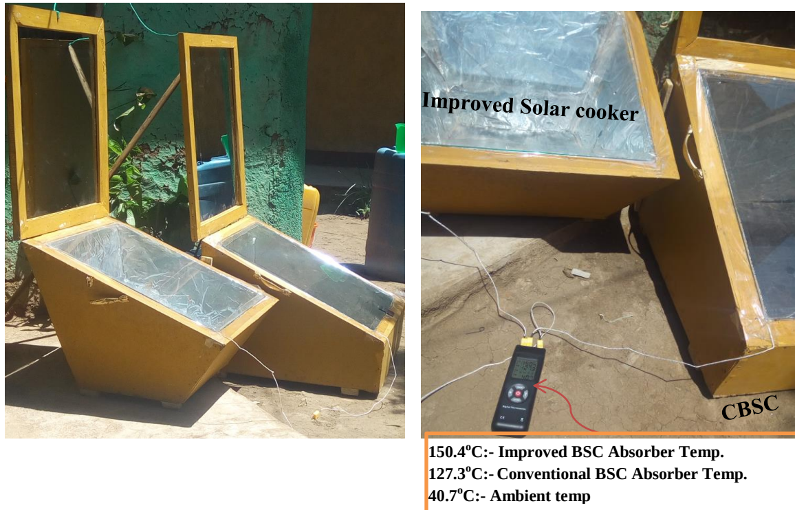
FIGURE 3-3: Experimental setup and during testing
