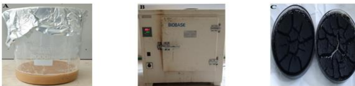
Figure 3.3. Activation of corncob: (A) powder of corncob soaked by 85%v/v of phosphoric acid before oven dry; (B) oven drying at 120°C for 12hr and (C) the soaked corncob powder after oven dry.
