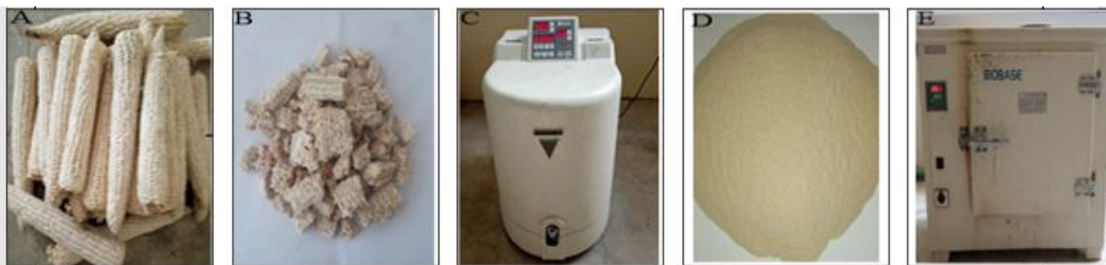
Figure 3.2. Row corncob preparation: (A) the raw corncob before size reduction;(B) the cute corncob;(C) the size reduction using ball mill at 350rpm for 30min, (D) the corncob after size reduction below the 60mesh sieved and (E) drying corncob using oven at 105°C for 12hr.
