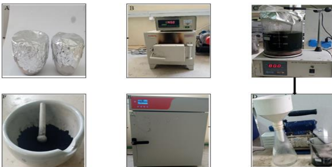
Figure 3.3. Activation of corncob: (A) powder of corncob soaked by 85%v/v of phosphoric acid before oven dry; (B) oven drying at 120°C for 12hr and (C) the soaked corncob powder after oven dry.
