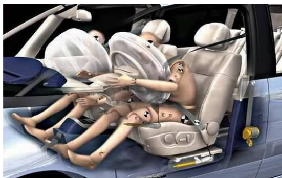
Figure 2. 11: Airbag (Wang et al., 2018)
