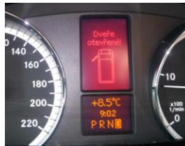
Figure 2. 9: Door warning (Safety, 2018)
