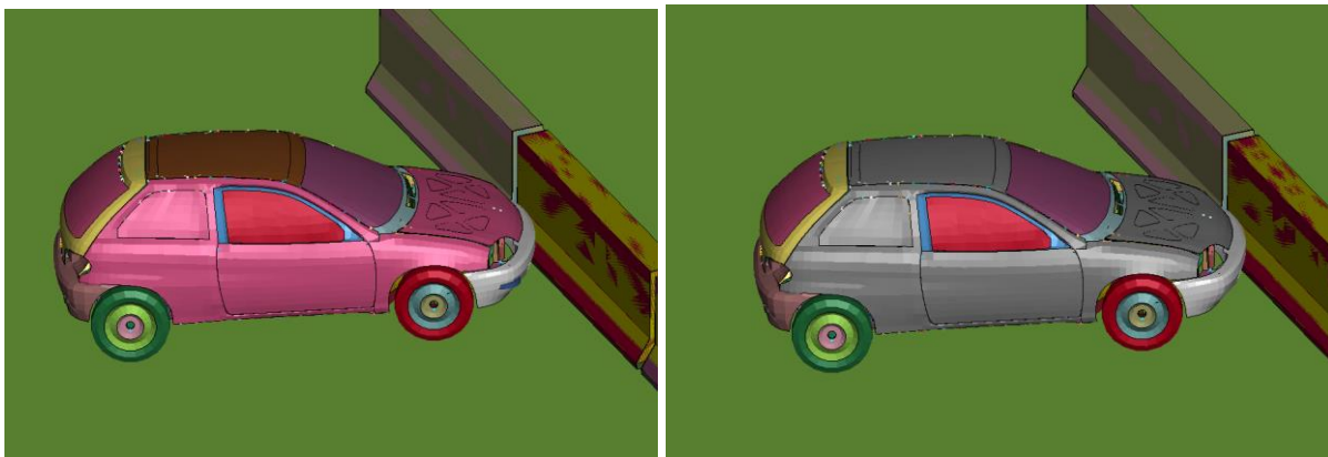
Figure 3. 23: Vehicle crash configuration at large collision angle
