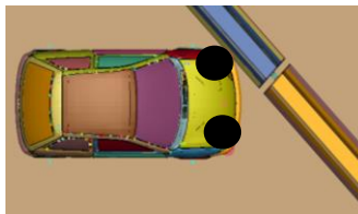
Figure 2. 21: First contact places during a non-perpendicular collision
