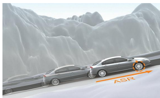
Figure 2. 3: Anti-Slip Regulation system (ASR) (Buznikov, 2018)
