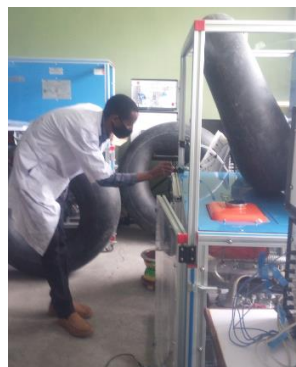
a. Adjusting Rotameter valve
