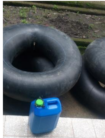
Figure E.1. During compressed biogas in a tire tube by using ordinary compressor
