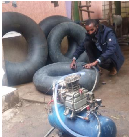
Figure E.1. During compressed biogas in a tire tube by using ordinary compressor
