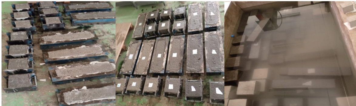
Figure 3.10: Casting and curing specimen.
