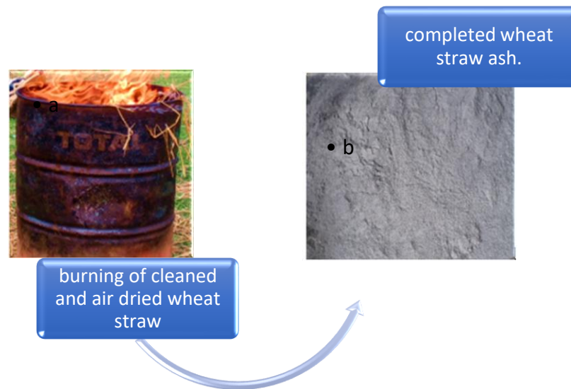
Figure 3.5: The process of preparing wheat straw ash.
