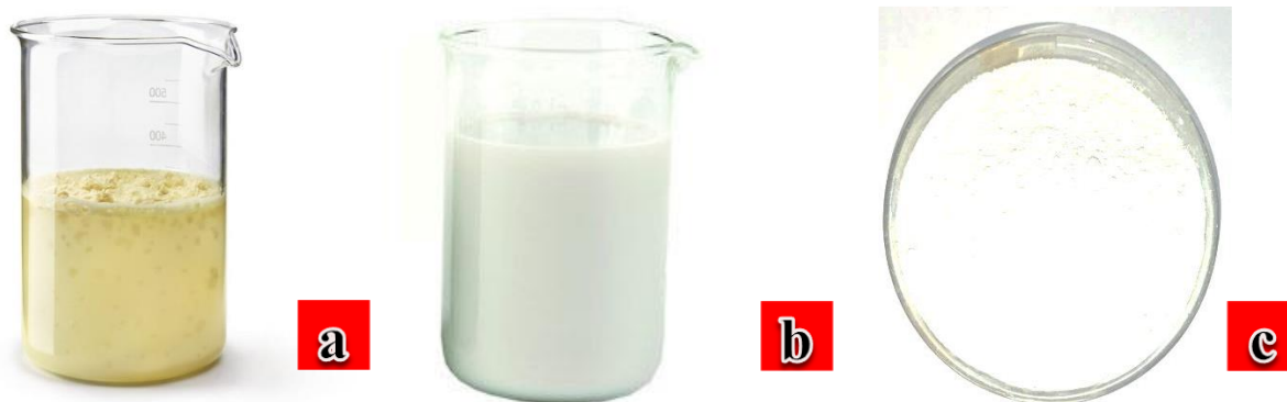
Figure a) Washing using HCl b) Washing using water c) Oven dried CFW
