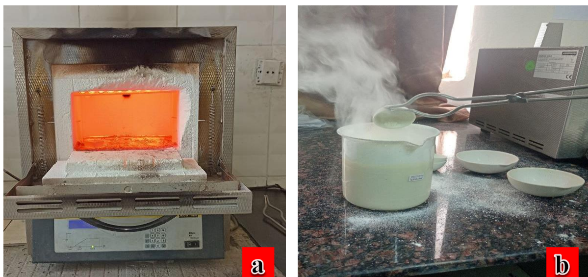
Figure a) Calcination of CFW with Muffle Furnace b) Immediate Quenching with Water
