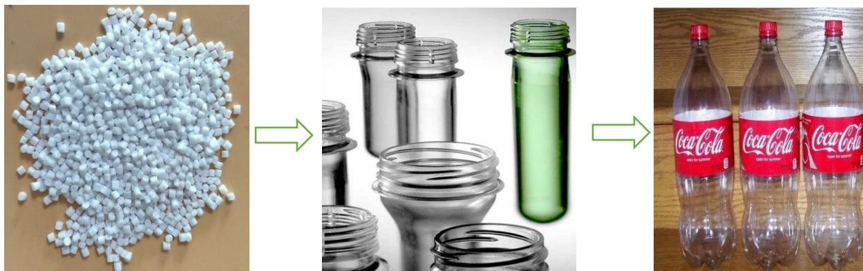
Figure 3.2 Formation of plastic bottle (resin, preform and plastic bottle)
