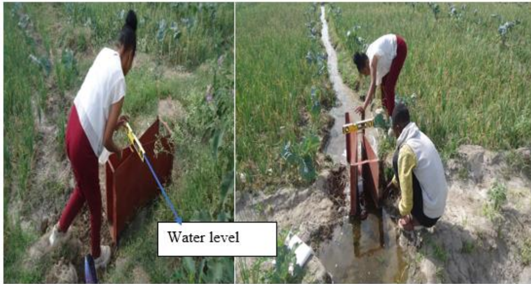
Figure 3. 3 Measurement of discharged at the farm using a 3-inch Parshall flume
