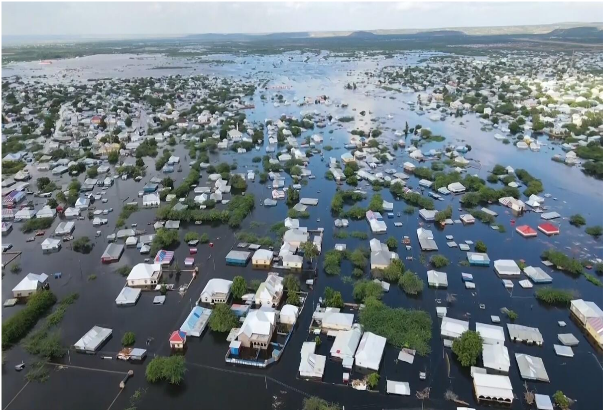
Figure 4.9: Aerial observation of the extensive flood inundation in Beletweyne, this observed reality serves as a qualitative benchmark for validating the spatial accuracy of the HEC-RAS simulated flood boundaries
