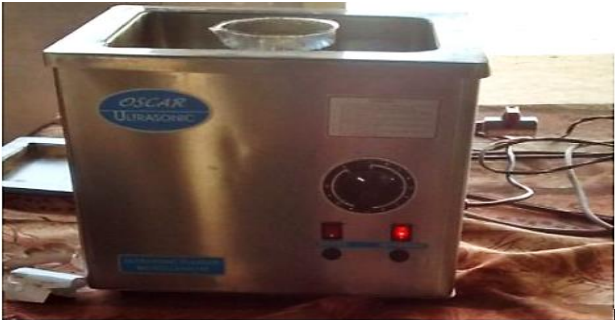
Figure 1.1 Nano fluid preparation, Ultrasonicator.
