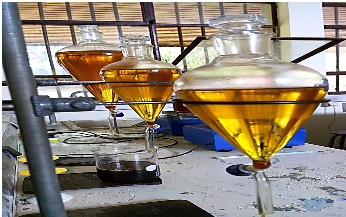
Figure 3.10 Separated glycerol and biodiesel before washing
