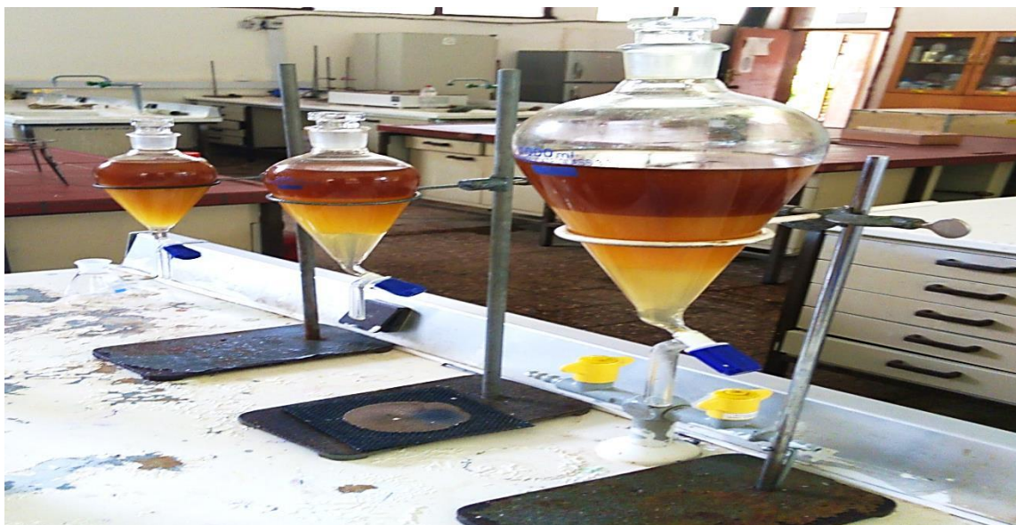
Figure 3.13 The second step of washing biodiesel
