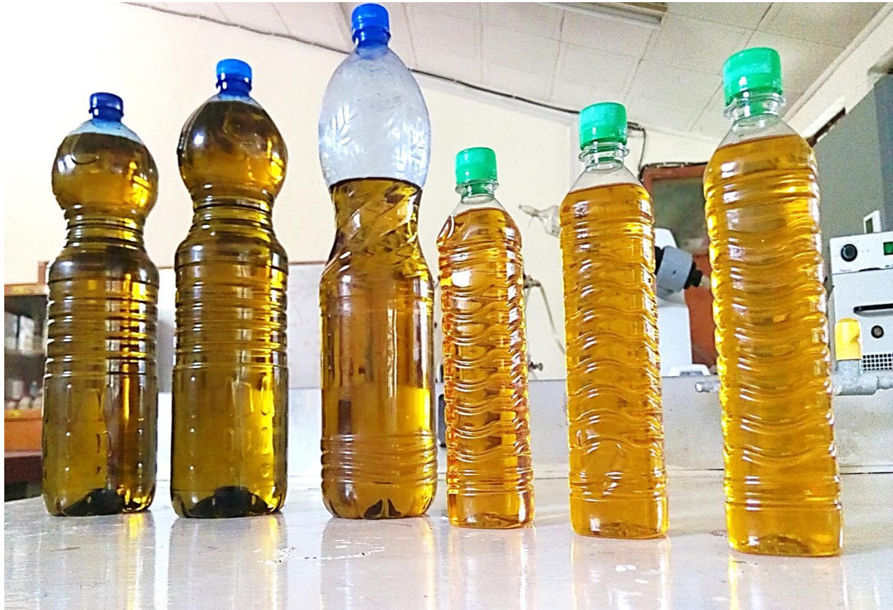
Figure 3.20 The final collected biodiesel and ready to use into the engine
