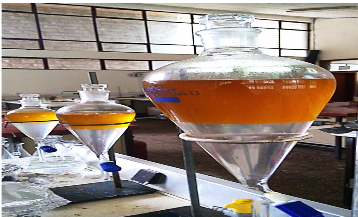
Figure 3.16 The fifth step of washing biodiesel
