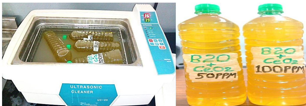
Figure 3.22 Ultrasonicator sated at a frequency of 40 kHz for 30 min.
