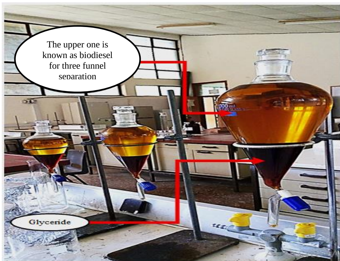
Figure 3.9 Separated glycerol from methyl ester (ME)
