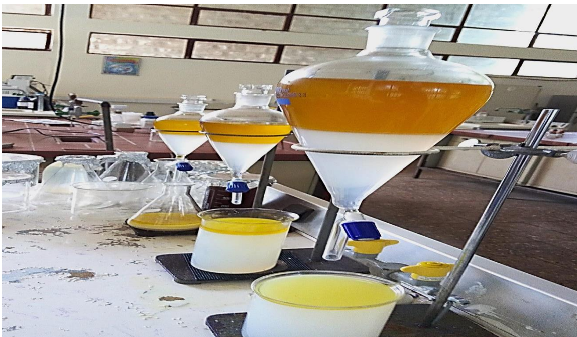
Figure 3.15 The fourth of step washing biodiesel
