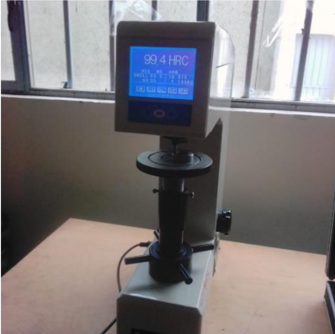
Figure 3. 10 Sample and Rockwell hardness tester setup
