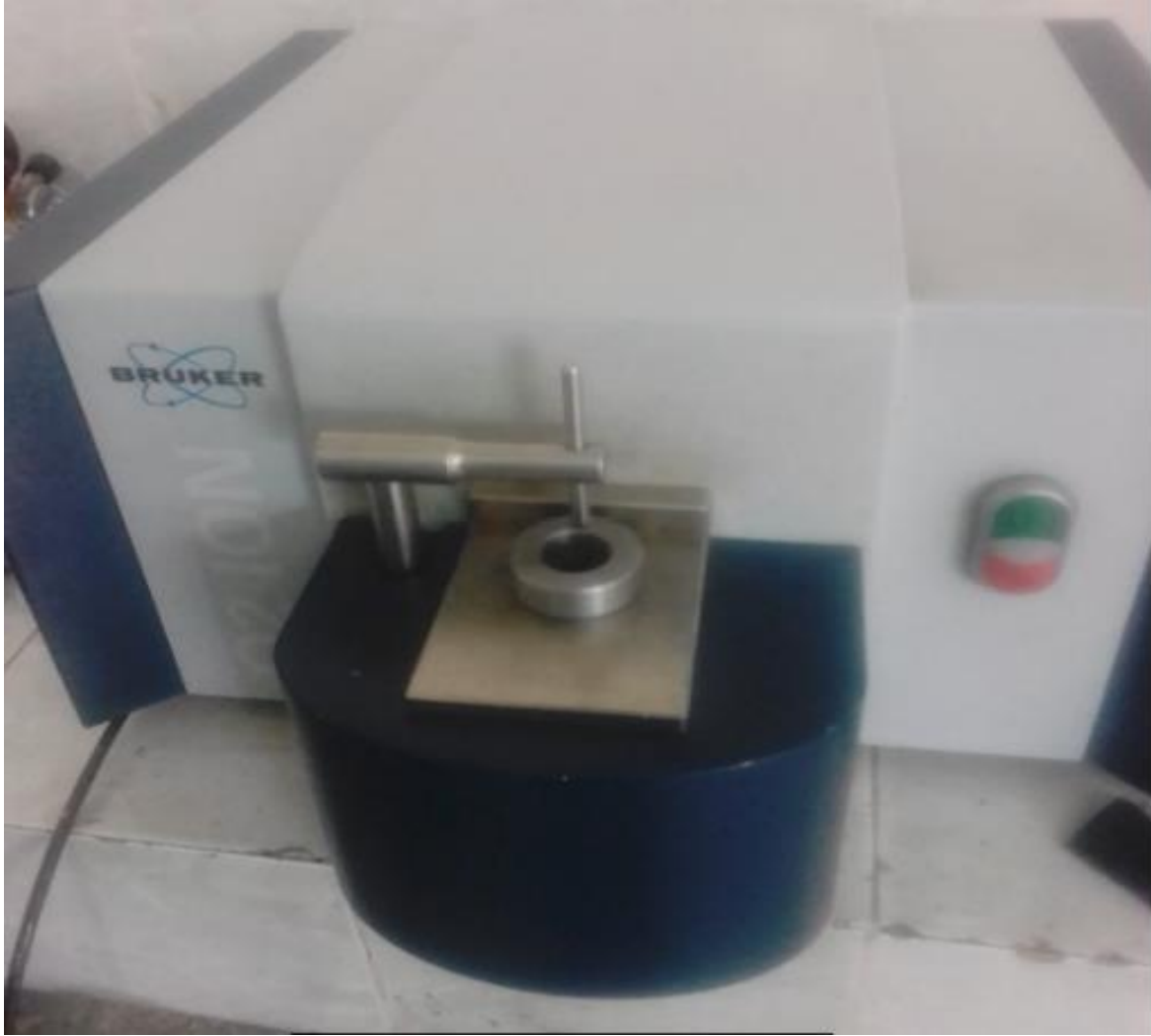
Figure 3. 9 Composition test for existing wheel from scrap
