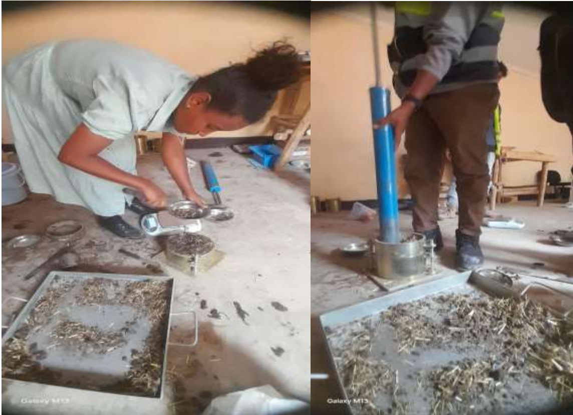
Figure 3.6: Photo while performing compaction test in the lab
