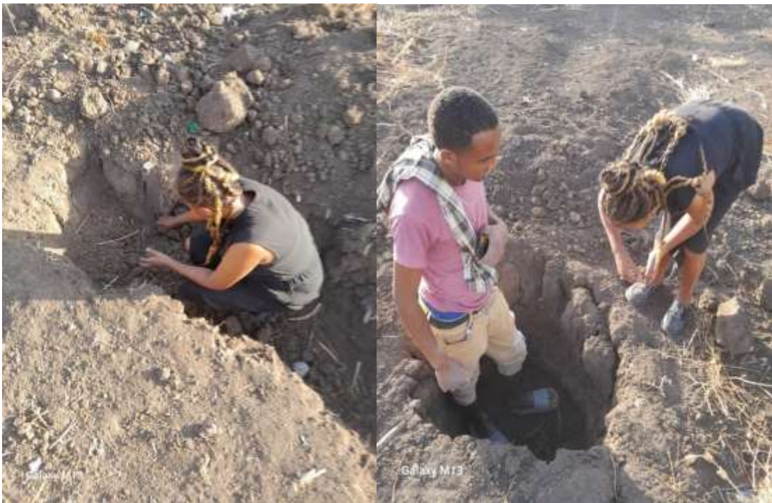
Figure 3.3: Sampling of expansive soil from test pit
