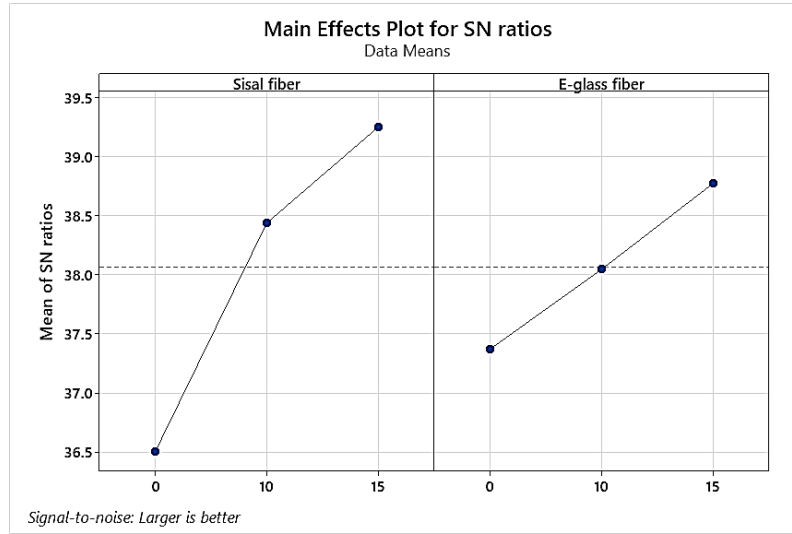
Figure 4. 9 The main effect plot for the SN ratio of the Vickers hardness
