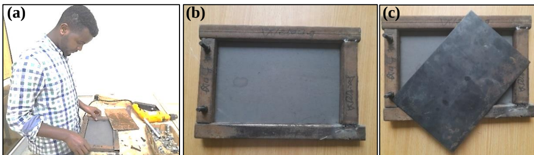
(a) Mold preparation in a shop (b) Prepared mold (c) Mold with top cover plate
