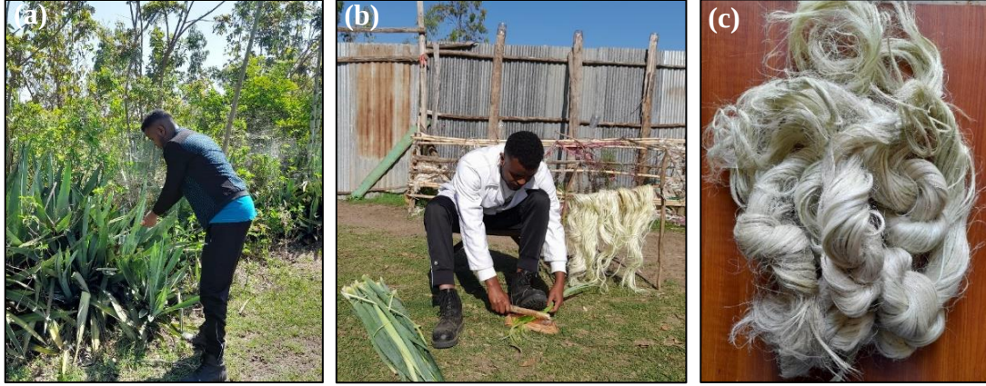
(a) Harvesting sisal leaf (b) Manual extraction (c) Extracted sisal fibers
