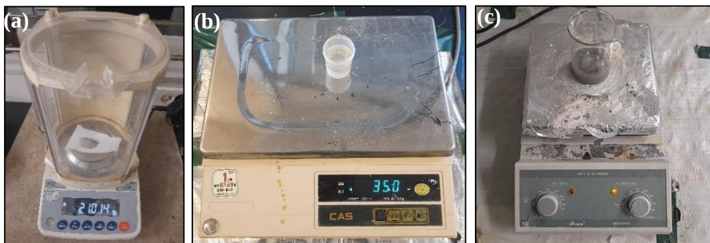
(a) Measuring SiC filler (b) Measuring adhesive material (c) Mixing filler with adhesive
