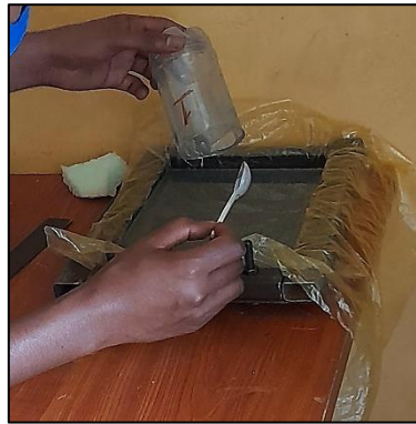
Figure 3. 16 Hand layup process
