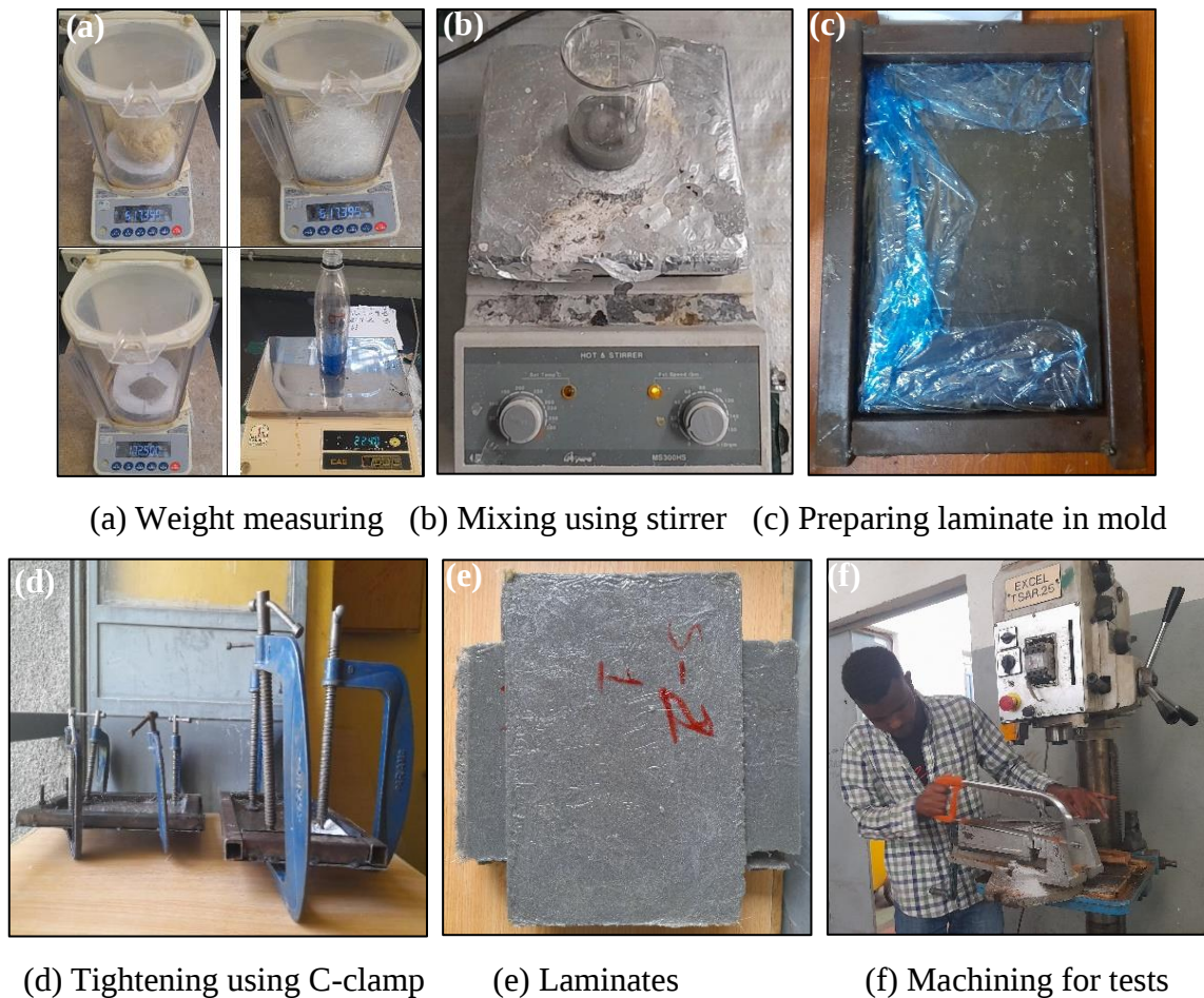
Figure 3. 18 Composite fabrication process
