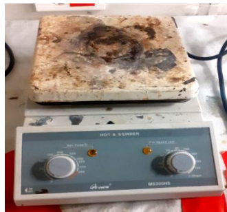
Figure 3.15 Magnetic stirrer & hotplate MS300HS.
