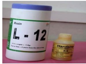
Figure 3.1 Epoxy (L-12) and hardener (K-6).
