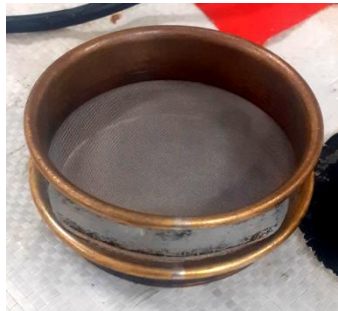
Figure 3.14 200 Mesh size Testing Sieve.
