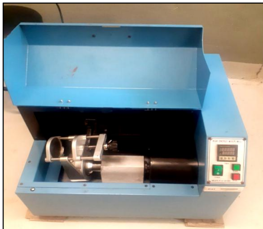
Figure 3.13 High energy mixer/mill.
