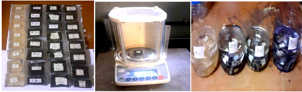
Figure 3.24 (a) Water absorption specimens (b) measuring weight before and after immersion (c) Specimens immersed in water.
