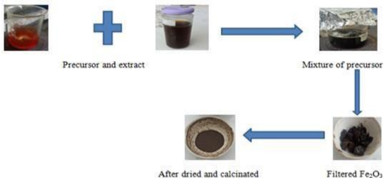
Figure 5: Schematic diagram of synthesis process for Fe 2 O 3 nanoparticles
