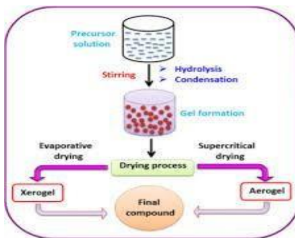
Figure 2: Sol-gel method processing (Ganachari et al., 2019)
