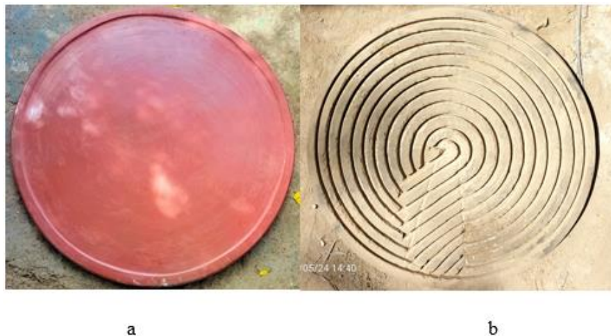
Figure 5.1 a) Smooth top surface and b) Grooved bottom surface of the mitad.
