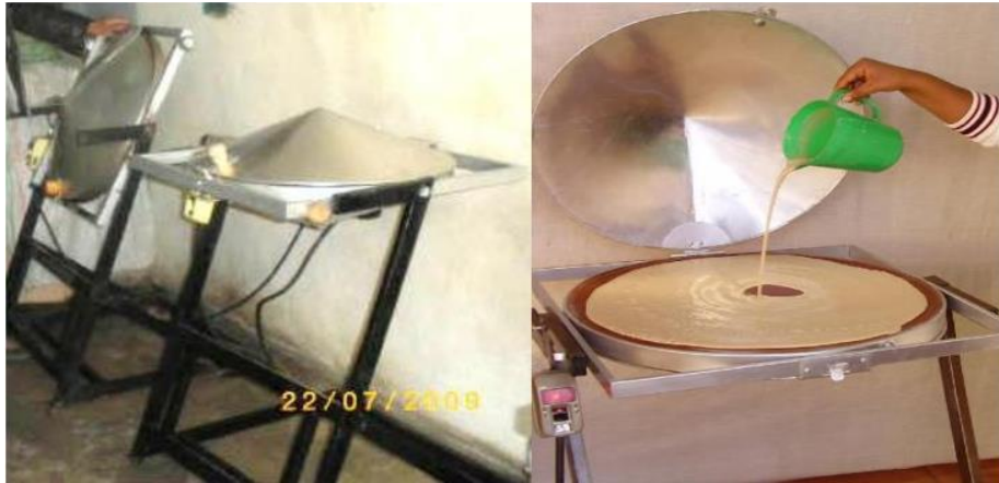
Figure 2.8 Double sided electric injera mitad (Yesehak, 2019).
