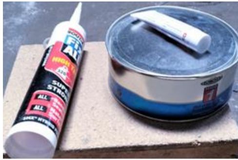
Figure 5.5 Polyester putty bonding material
