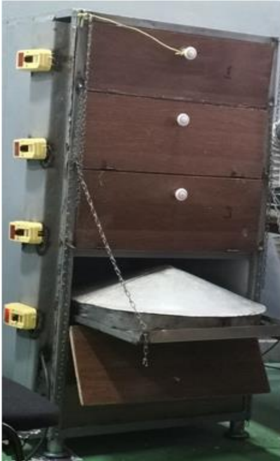
Figure 5.10 Assembly of multi mitad injera baking electric system
