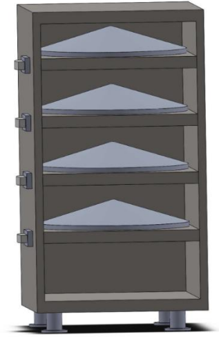
Figure 4.4 Conceptual schematic diagram of injera baking electric mitad assembly.
