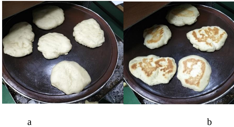
Figure 6. 15 Actual bread baking tests of the electric mitad a) Dough on surface of mitad b) Baked ready bread
