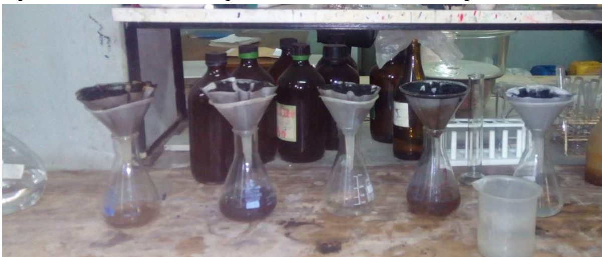
Washing prepared ACs using 0.1N HCl and distilled water
