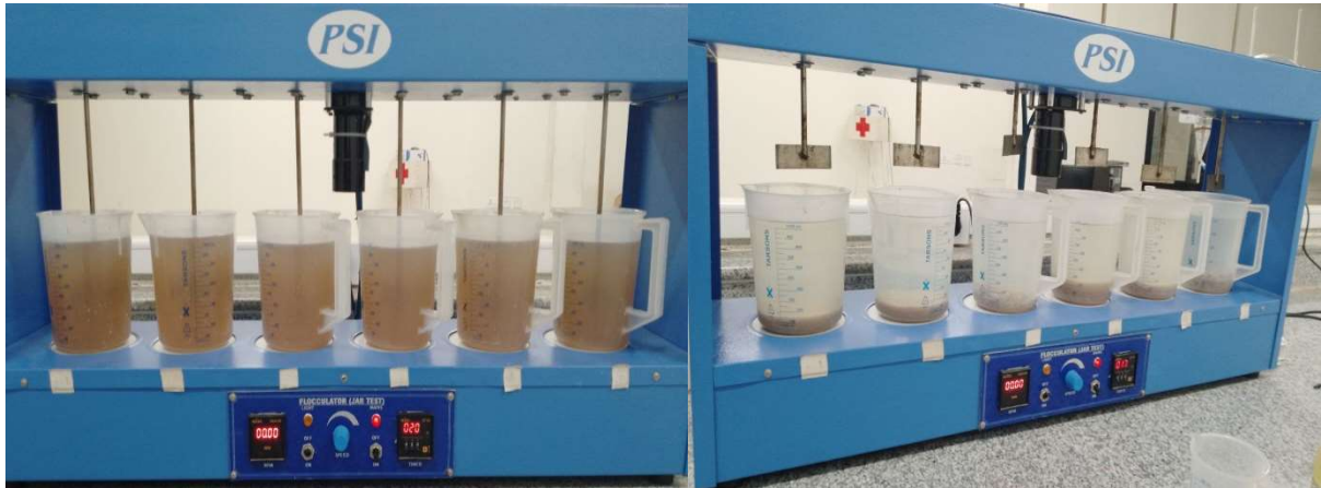
A. Photographic representation of before and after treatment of textile wastewater
