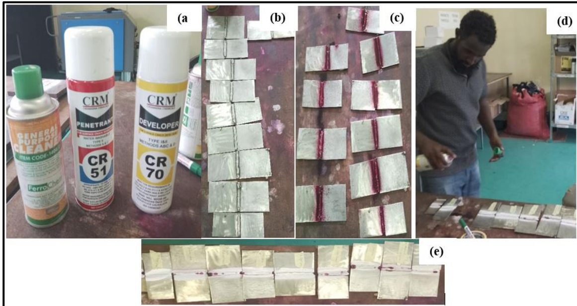
Figure 3.13: PT process: a) cleaner, penetrant and developer chemicals b) pre cleaned samples by using general purpose cleaner c) the use of penetrant fluids d) the use of developer e) examination of the test surface
