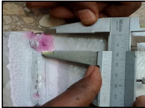
Figure 3.12: Surface defect measurement after LPT
