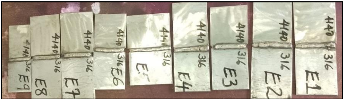
Figure 3.10: samples after welded
