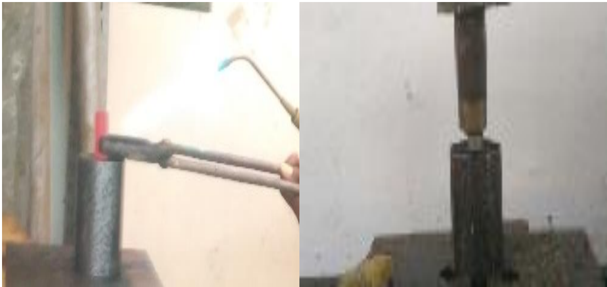
Figure 3.7 Hot extrusion set up during operation
