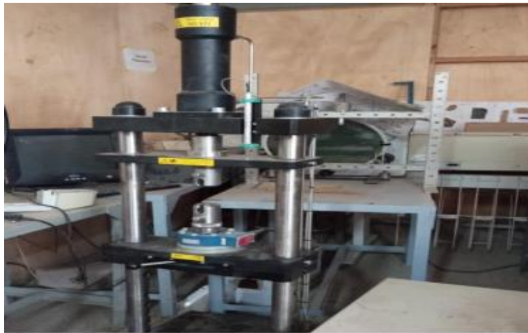
Figure 3.11. Universal testing machine setup used for compression test
