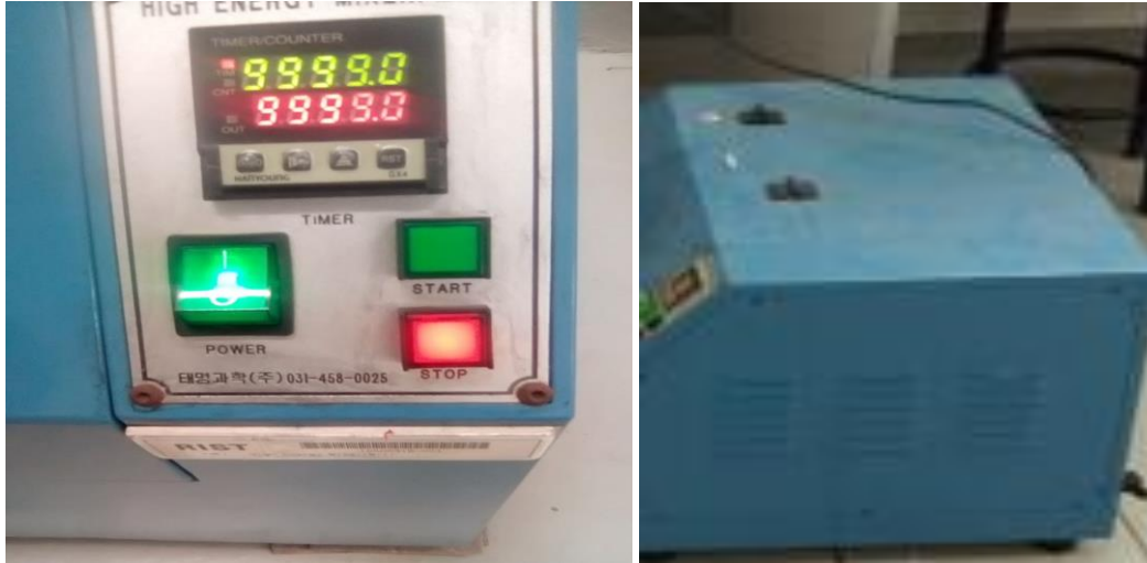
Figure 3.3. High energy planetary ball mixer used to mix the powders.
