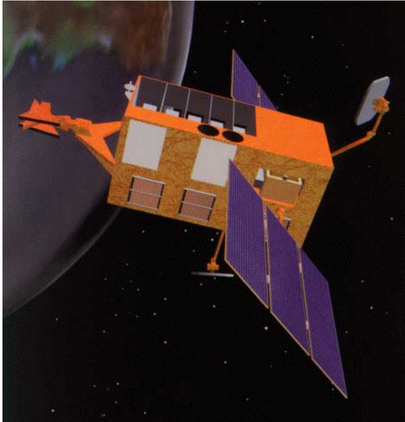
Figure 3.1: NASA's RXTE satellite with ASM, PCA, and HEXTE instruments. Source: NASA (1996).
