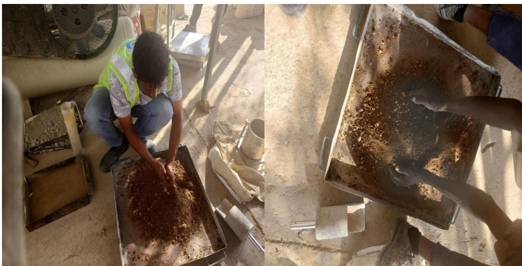
Figure 3-12 modified proctor test
