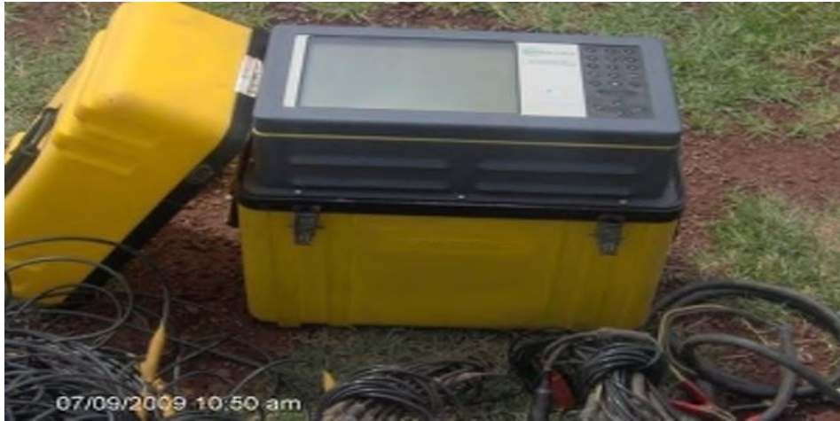
Figure 3.4: Smart Seis of Geometrics of USA
