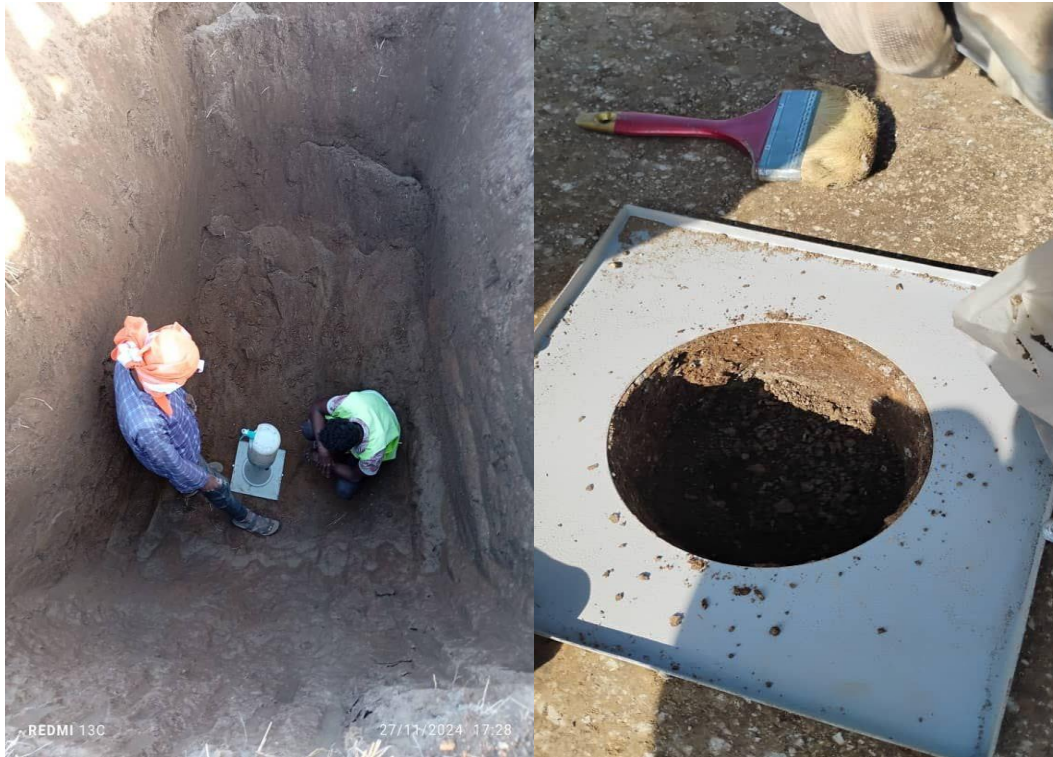
Figure 3-16 Field Density Test (FDT) by Sand Cone Method
