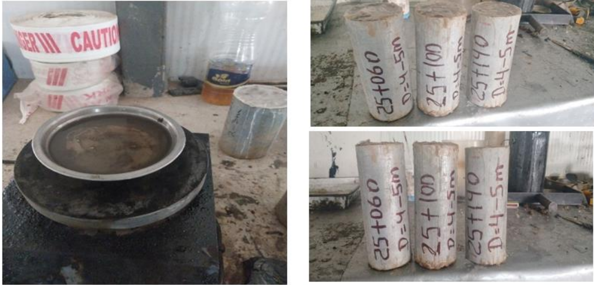
Figure 3.10 sample preservation using wax
