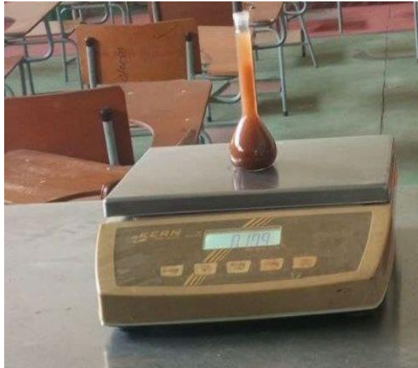
Figure 3-11 specific gravity of soil
