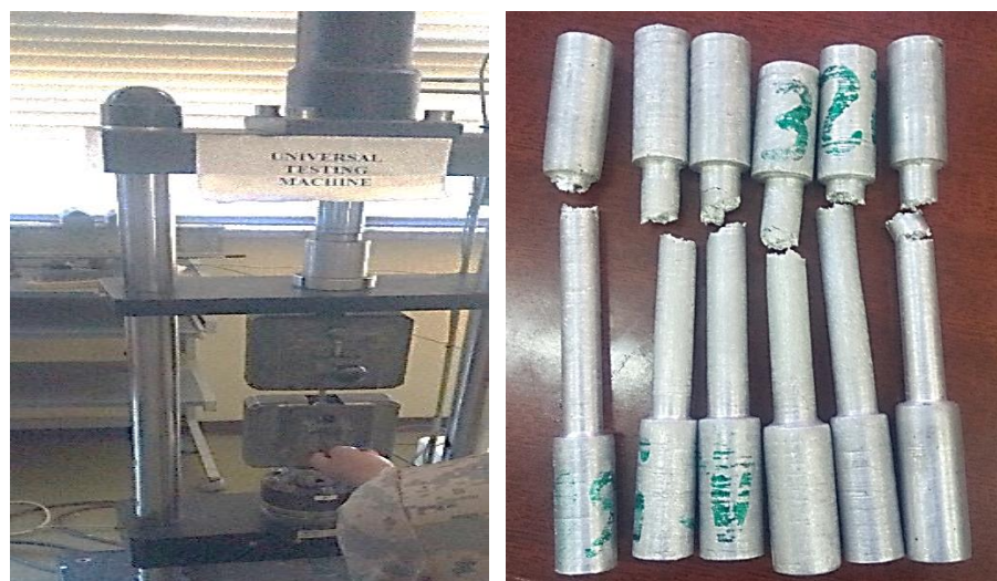
Figure 4.3 (A) Tensile test set up on UTM (B) plastically deformed tensile test specimens.
