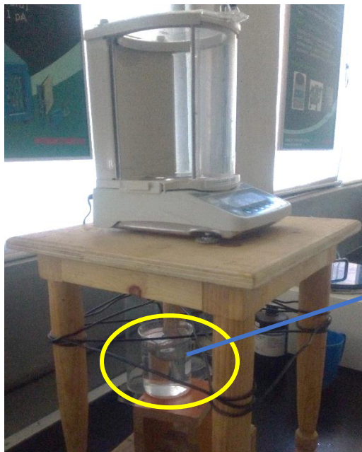
Figure B-.0.4. Setup for measuring mass in distilled water
