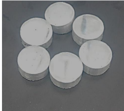
Figure 3.14 Microstructural and hardness test specimen 20 mm diameters with 10 mm height
