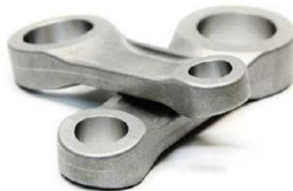
Figure 2.3. Connecting rods made of Al-Al 2 O 3 (Przemyslaw and Aleksander, 2013)
