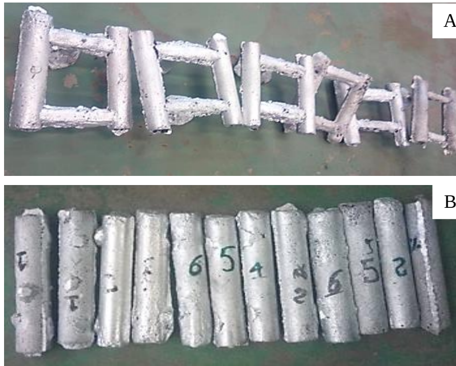
Figure 3.9. Solidified cast hybrid composite specimen (A) before runner, riser and sprue is cut out (B) after runner, riser and sprue is cut out
