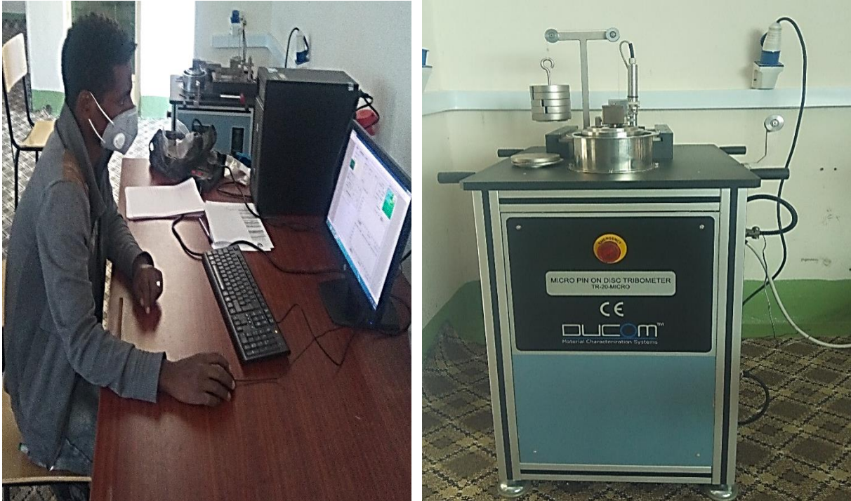
Figure B.0.8. Full image micro pin on disk tribometer use for wear test.
