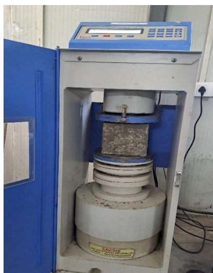
Figure 11 Compressive strength test machine at LEA-LASA Engineering consultant laboratory.
