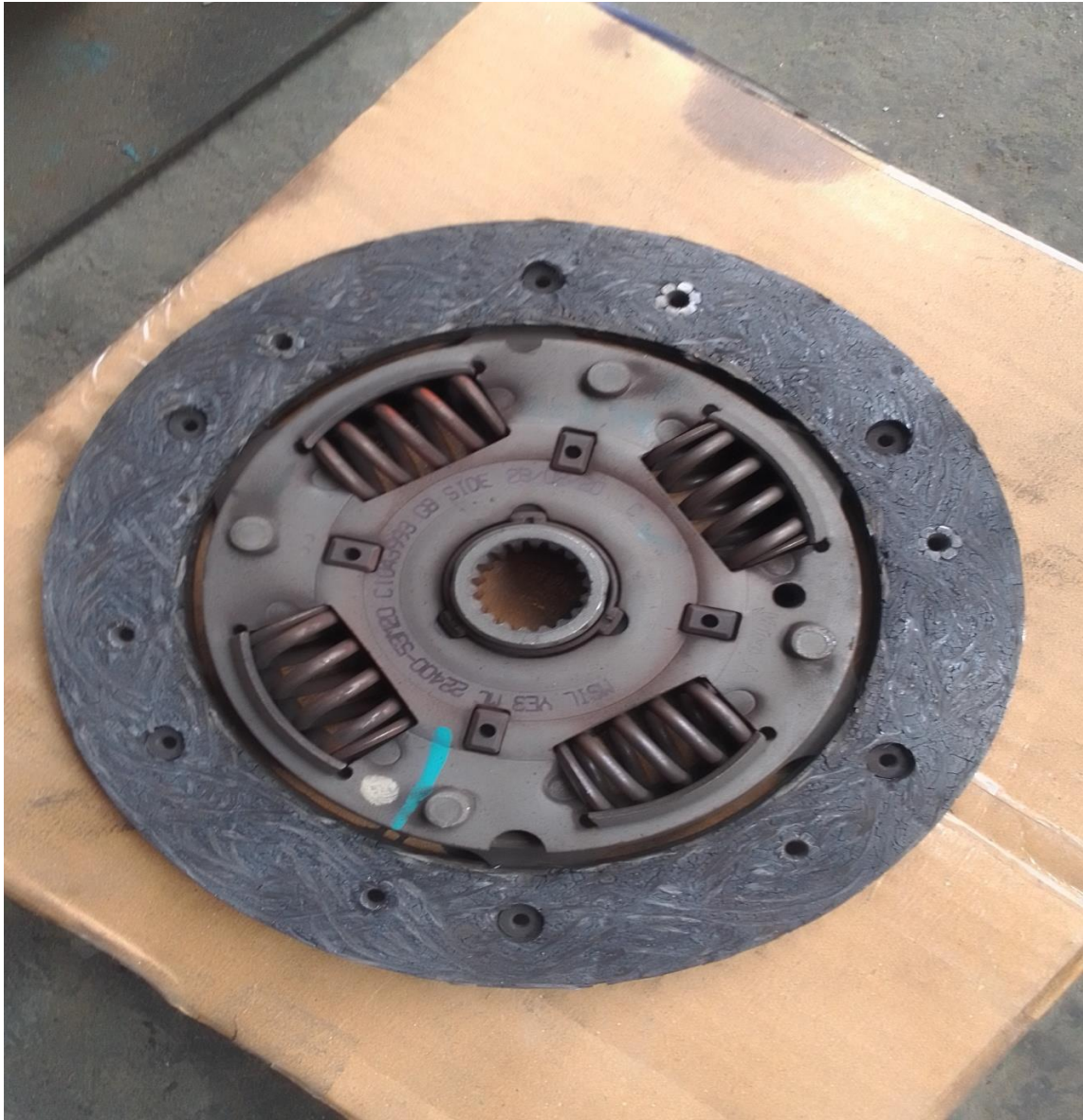
Figure 1.2 Premature clutch plate failure due to thermal load
