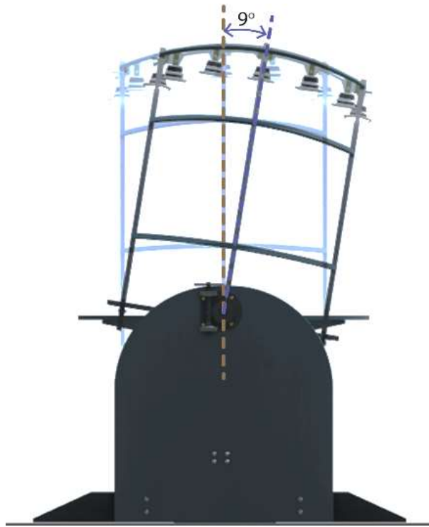
Figure 45 Heliodon locked at 9 ° latitude for solar analysis
