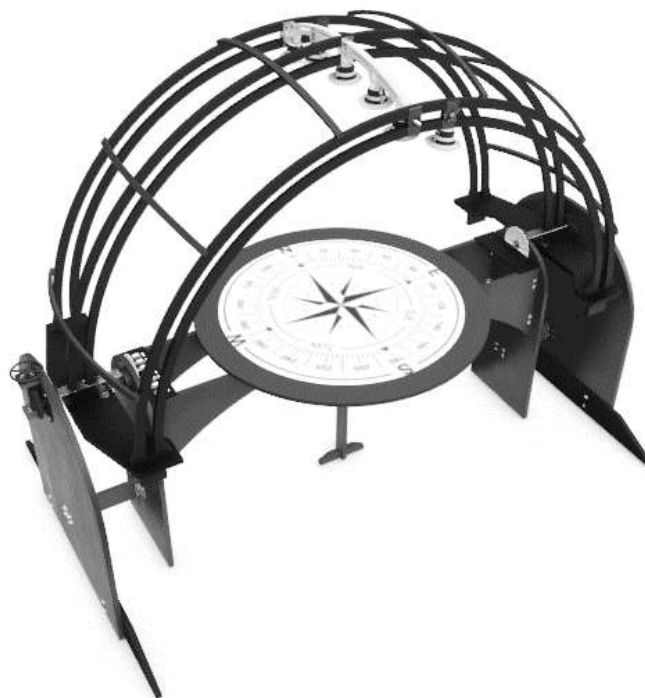
Figure 38 Custom-made adjustable Heliodon
