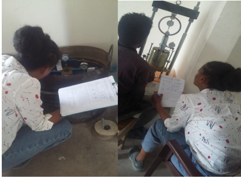
Figure 20: CBR test done at BEAEKA laboratory
