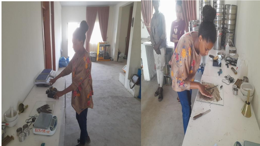
Figure 18: Atterberg test done at BEAEKA laboratory
