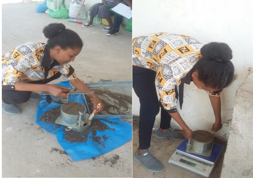
Figure 19: Compaction test done at BEAEKA laboratory
