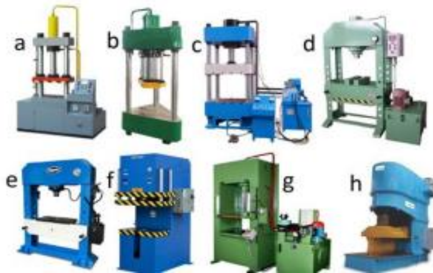
Figure 2. 1. Various types of hydraulic press frames (a) Two Column Press, (b) Three Column Press (c) Four Column Press (d) Fabricated Four Column Press (e) Fabricated Two Column Press or H-Frame Press (f) C-Frame Press (g) Close-Frame Press (h) Fabricated Chamber Press.
