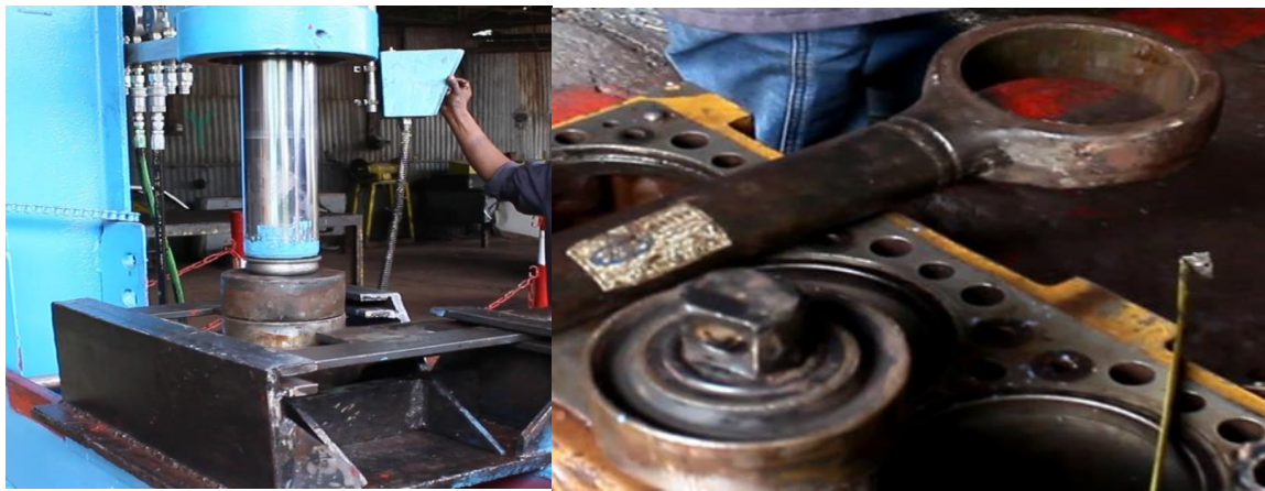
a) Assemble and dissemble process of torque rod b) Disassembling of torque rod bushing
