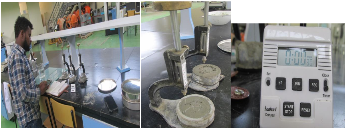
Figure 3: Setting time of cement paste
