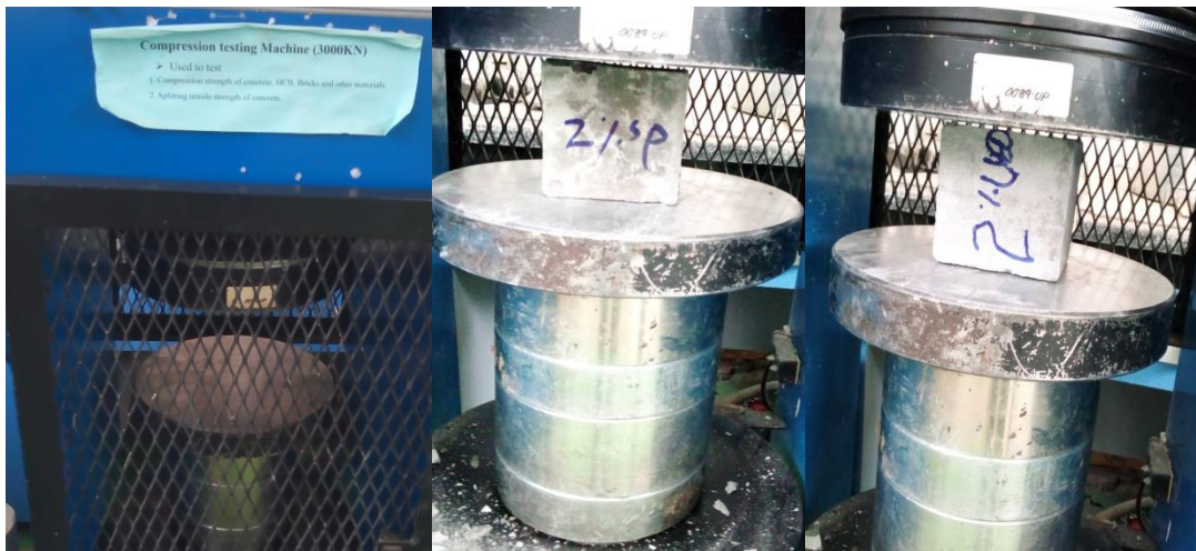
Figure 3.6 Compressive strength tests after 28 days
