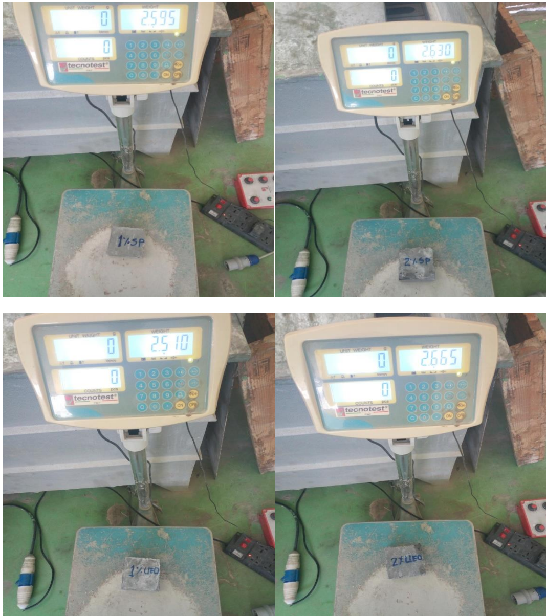
Figure 7: Weight of samples after immersion
