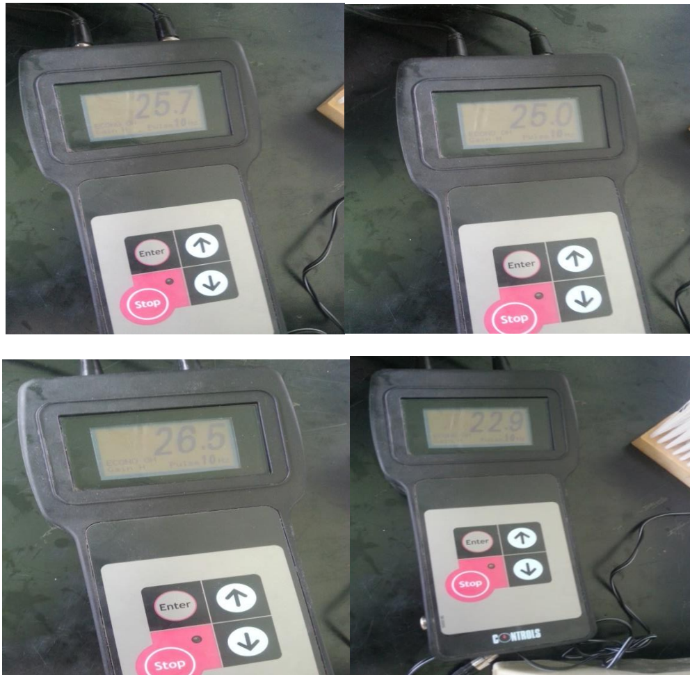
Photo of time of traversing recorded in microsecond for mixes
