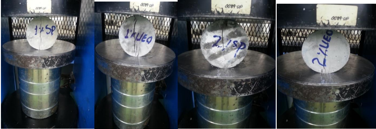
Figure 3.7 Split tensile strength test at 28 curing days
