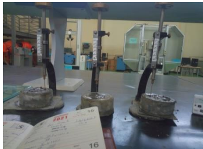
Figure 3.2: Vicat apparatus for setting time test of normal consistency of cement paste
