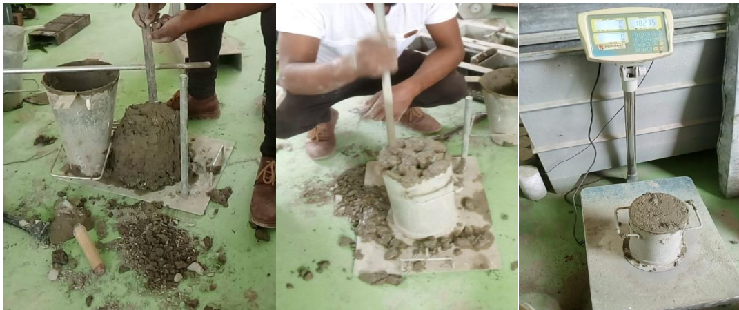
Figure 3.5 Slump and compaction factor test
