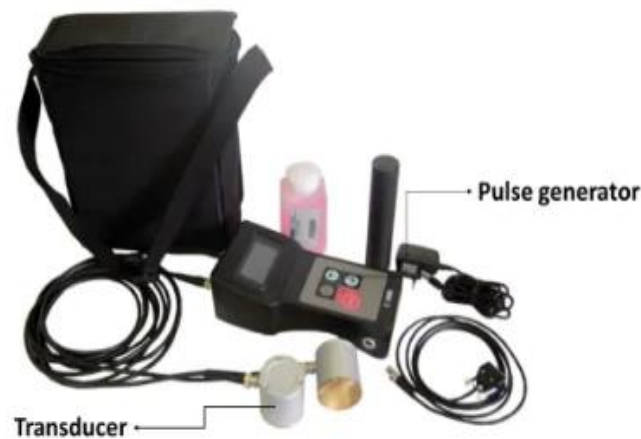
Figure 3.8: Ultrasonic pulse velocity test instrument
