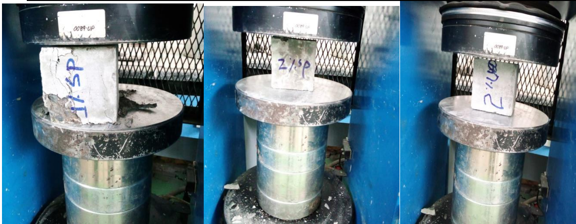
Figure 6: Compressive strength test
