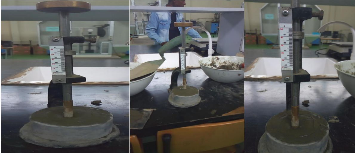
Figure 2: Normal Consistency test
