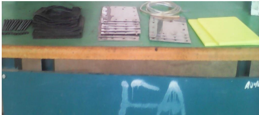
Figure 3.1 materials used to build HHO gas dry cell
